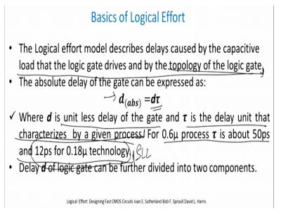
As you can see the logical effort model describes delays which is caused by capacitive load that the logic gate drives and the topology of the logic gate and I will explain to you what these what these two things are it means to say that.
