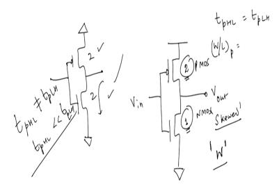
If you remember we had learnt in the our earlier modules that if you have a simple transistor CMOS transistor right CMOS transistor then if you have a MOS device and you have an NMOS here and this is your V out right and this is your V in then we have learnt that for the design to have equal delays which means that to have that tpHL = tpLH require a W/L ratio of PMOS should be approximately twice the W/L ratio of NMOS right.
