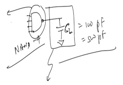
If you have let us suppose you have gat right and then the gate is driving some external logic right external logic whose value is CL right then this value of CL load capacitance will actually
