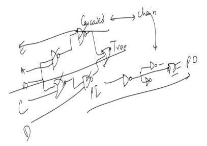
And that two methods are known as you will have one method which is basically a cascaded method right cascaded method but this is basically a chain method so you will have a chain available to you can also have a tree method right which means that chain is something like this that you are able to drive a something like this right so will have chain of devices being attached
