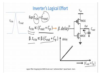
So assuming that your input rise time which is basically my this one trin is the input and tr out means rise. So trin basically means that the current is coming into the system right and that time the value of current coming from 10 to 90 % is basically varying from 10 to 90% is basically my input current and when the output side the current of the voltage is falling from higher value to less than 10 volts or 10 milli amps we get what is known as a r out delay out right fine this is what we get.
