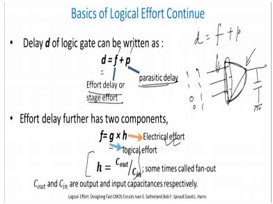
So I will just see what is these two components are the two components which we referred to delay of a referred to is written as D = F + P where F is defined as the effort delay or stage of a and P is the parasitic delay. So we define D which is basically your logic gate delay is nothing but a some of F and P where basically P is the parasitic delay and F is the effort delay or stage effort I will explain each one of them individually before we move forward.
