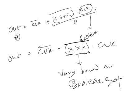
So you see out is defined in this manner out is defined as right I will just switch it is clock bar + is defined as clock bar + A right dot B + C bar of that into clock. So whenever your clock is high evaluation phase this becomes 1 depending upon the value of ABC this becomes high or low therefore it becomes we will get an output.
