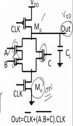
So this is the last part which I was trying to say that (once the out node is charged similarly once the output node is discharged there is no other way to charge it until and unless we reach the next recharge cycle are you able to get the picture. That once we until and unless we get into the next cycle once discharge cycle once discharge is gone. So the data once it was stored in the CL Me becomes high your PDN is active and the output goes to 0 and you finished.
