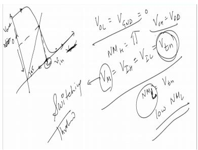
One more thing in this case is that VOL will be equal to VGND ground which is 0 approximately output low and the reason is that you are allowing the voltage at the output node to go to the ground node right and it is going very easily like obviously it will go very fast because you have high current to flow there and as a result it will always go to ground load.
