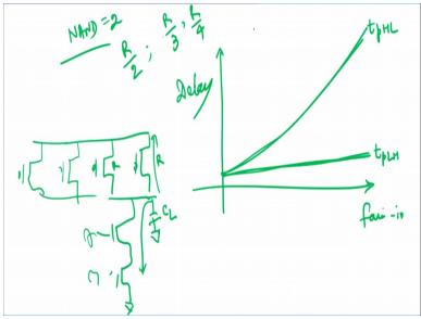
That let us suppose I have a NAND gate right I try to plot your fan-in and I try to find out the value of tpHL and tpLH then this is how it looks like. This is tpLH and this is tpHL this is for NAND 2 logic right and this is the variation of so this is your delay and with fan-in NAND if you remember was basically your pull up was basically your 2 PMOS is parallel and this is 2NMOS is in series right.
