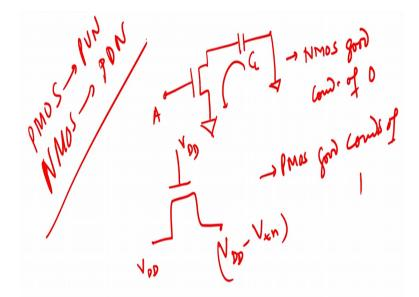
If an NMOS is a very good string passage of 0 right so you got NMOS inverter in the serial is charged to some value then this CL will discharging here and the voltage here will be starting to fall down at the particular point now NMOS inverters are good conductor of 0 right. And PMOS are good conductors of 1 which means that whenever through an NMOS and 1 is past between input and output of NMOS.
