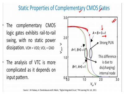
Let me come to therefore the static properties of the complementary CMOS gate right static properties means what? I will take a 2 into so is this example is taking input NAND gate right. So input NAND gate I just not draw here and I will draw it for you again.
