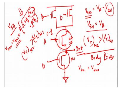
Let me explain to you in that sense that I have again simple inverter appear here right and this is grounded so this is A right this is M2 let us suppose and I have an internal load here INT let me name it I have M1 here and this this is B and of course this is A and of course this is B right. So I can write down VGS2 gate to source gate to source of 2 M transistors nothing but equals to VA is this one – VDS1.
