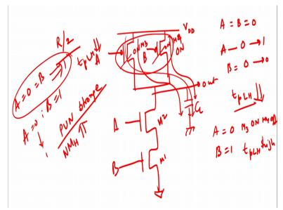
That I have got a VDD supply here right and then I have got this and I have got this then I have got 2 NMOS's in series to each this is A this is B and I have got PMOS's in parallel to each other this is A this is B and output is taking somewhere from here right. So what I wanted to show to you is that when you have a CMOS inverter right CMOS complementary CMOS inverter.
