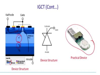
So, this is the device structures cathode and anode and you know this is actually n buffer region, it is doped in such a way it does not offer a very high on state resistance and in between there is actually silicon, silicon doping level is prescribed by the colour, this is the highest doping level and this is the lowest doping level via distance and this is the actually symbol of this device, you have a gate cathode, anode.
