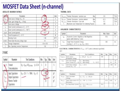
So, VDS can be 500 volt but where we are talking about 1000 volts and more than that so, drain to source voltage will be this and VGS voltage source will be +-30 and ID for 25 degree centigrade, it can be around 10.6 ampere, so for the 100 degree centigrade, it has to be derated, so it has to be this much and 10 current, if it is pulse kind of waveform, so it can be as high as a 42 amperes and these are the data sheets you have to design, we will show it how to design.
