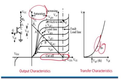
This characteristics same as the characteristics of the BJT which you have studied in the normal BJT applications in your analog electronics, so this is your load line and this is the IC and VC and this is for the different kind of instead of IB, you will have the gate voltage, this is the only change, so you will have this trans conductance, so for this is, this is the actually power line and accordingly, you will have a VG which is for the current IC for the different values of VG.
