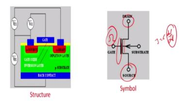
So, this is the structures of the MOSFET, we have actually VDS that is tend to source voltage and we call drain and the source generally high voltage site is said to be the drain and other site is said to be the source and we have GS that is a connected between this actually source and the gate and what happened you know actually this is called drain and this is called source, then it can be actually different kind of MOSFET that is enhancement MOSFET, depletion MOSFETs.
