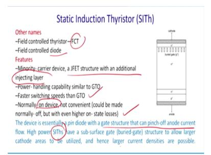
But problem lies you know actually its power handling capability is quite low, so another members of the thyristor is called static induction thyristors, so there actually it is field controlled thyristors or FCT or field controlled diode and it has a features like the minority carrier device, a JFET structures with an additional injecting layer is been provided by the method of induction.
