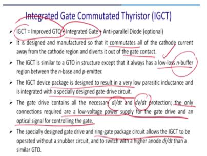
So, it is improved GTO and integrated gate that is the features of IGBT that essentially form BJT when you got an insulated gate that becomes IGBT, it is an actually a combination of the advantage of the MOSFETs and the BJT, here it is essentially a combination of MOSFET and GTO, so integrated gate and also insulated gate and anti-parallel diode, MOSFET I will take at last, so we shall understand it better.
