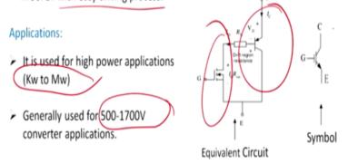
Now, let us come to the another important member of this power electronics that is insulated gate bipolar transistors, this invention itself is a mark of the change of the face of the power electronics, so Dr. Baliga, actually in G, General Electric discovered it and we are Indian, so we should be proud of his discovery, IGBT is preferred over the MOSFET because of its on state loss as compared to the MOSFET with a very easy driving process.
