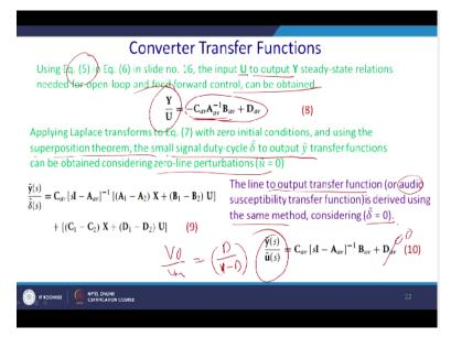
So using this equation 5 and 6, please refer to this equation 5 and 6 because I will be recalling. So this is the 5 and 6 because this is the steady state DC values. The slide number 6, the input U to the output Y steady state relations needed for the open loop and feed forward control, can be obtained. That is the transfer function, that is the output/input. So same thing we can get if we have, if you know this basically the A matrix C matrix and the B matrix.
