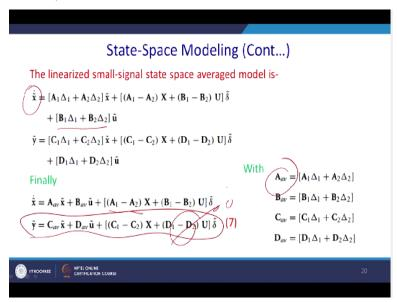
Thus we can linearize with that help and ultimately  $x\sim$  can be actually substituted, those terms which can be equated to 0, ultimately A1delta 1+A2delta 2+x A1-A2X B1-B2\*U to delta and B1\*delta 1+B2\*delta 2\*u. So there should not be any term without ~. So all the DC value has been eliminated from the overall equation.
