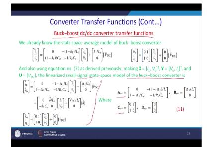
Now let us see Buck-boost converter transfer function. So you have written this matrices previously. So you can combine by this equations, also using this equation 7 derived previously making X is basically the current through the inductor and the voltage across the capacitor as V0 and essentially y is you can take it V0 as well as IL and U=of course, it is the input VDC.
