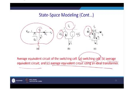
So ultimately you go back to your buck-boost converter. This is actually the switching configurations. So you got a switch and thereafter diode and you got an inductor here. So this should be on and off depending on the duty cycle and that actually the duty cycle is delta 1 and is the current control source, so that will be equal to I\*del 1. Similarly, it will be a delta1\*Vs but potential difference at this point is Vs, it is blocking the voltage Vs.
