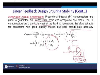
Proportional-integral compensator are used to guarantee steady state error with acceptable rise time. The PI compensator are a particular case of lag-lead compensator. Therefore, suitable converter with good stability margin but poor steady state accuracy can be achieved. So this is actually PI controller. So 1+sTz/sTp. So you can split it like that and you can rewrite as Kp+Ki/Ks. Or you can write it this term.
