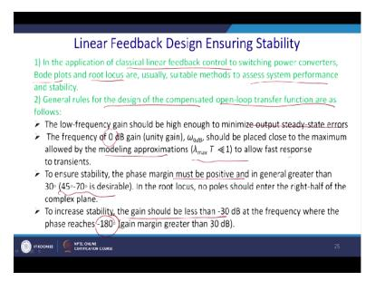
Now what we want basically the system to be stable first of course? And that is what we do. In the applications of the classical linear feedback which you have studied in your control system to switching the power converters, so we have while he was telling us the Bode plot, root locus, polar plot, Nyquist are usually suitable method to assess the transfer function. Now you got a transfer function and you have a Matlab, so it is very easy to analyze now a days.
