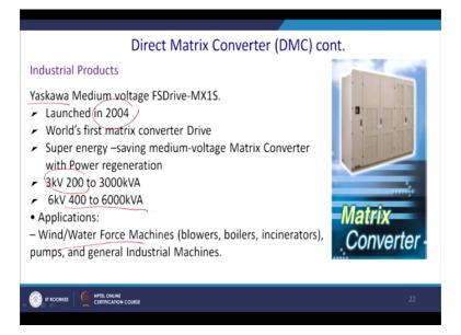
Now we can show this already been put into the industrial applications of the matrix converter. I am showing pictures of Yaskawa medium voltage FS drive MX. So it is launched you know around 14 years ago in 2004 world's first matrix converter drive. So it has been observed that super energy saving medium of the voltage of the matrix converter with power generations that is to the level of 3 kV to 200 volt.
