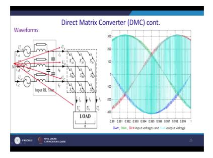
Now see that how we will generate different voltages. UAN, UBN and UCN are the input voltages and output voltages are U small a N. So you will be triggering in between quite high frequency because it was thyristors you are not allowed to trigger, you were allowed to conduct for an alpha of 15 degree, 20 degree, 30 degree but you can switch very accurately and generate the shape of the voltage as required.
