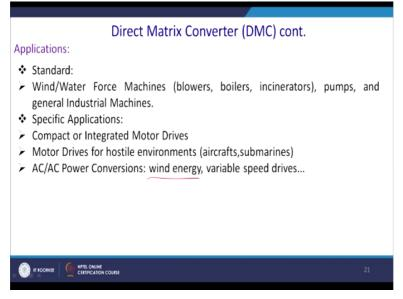
Now what are the applications? There is a wind applications, water force machine blowers, boilers, pumps and general industrial machines. Specific applications like compact and integrated motor drives. Motor drives for the hostile environments and also where mass or the
