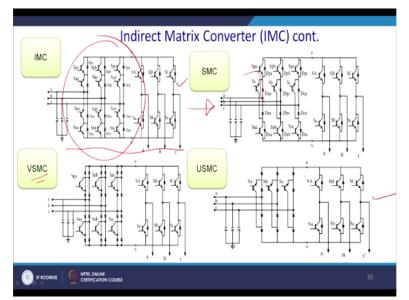
So that is the one of the challenge. You see that this is basically direct matrix converter, it is basically VMC, sparse matrix, it is SMC it is UMC. So see that a different configuration in a diode has been done. Since you want to make current so all the attention was paid to reduce the number of switches. So here is a normal IMC so this part is a three-level normal rectifier but without the DC link and two level inverter.
