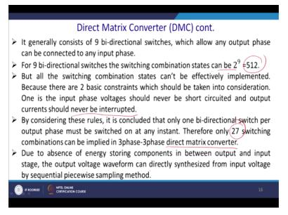
Nine bidirectional switching combination of states you know can have high rate of redundancies. So you can have as high as 2 to the power 9 combinations that leads to actually 512 combinations. So we require to understand that but all the switching combinations states cannot effectively implemented because there are two basic constraints we should be taken into the consideration.
