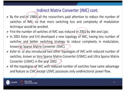
So few interesting features of this matrix converter indirect matrix converter, by end of the 1980s all the researchers paid attention to reduce the number of the switches of the indirect matrix converter. So that more switching losses and the complexity of the modulation can be avoided. First the number of switches of IMC was reduced in 2001 by famous scientist that is Wei and Lipo.
