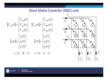
And so this is the actually the output voltage matrix and it is not that actually you can have asymmetrical configurations, mostly it can be used for the multiphase more than three-phase electrical machines, five-phase, six-phase. So you can have a more number of output legs also, that is also possible. So you have UaN, bN, cN and this is basically the output voltage matrix and you have input voltage matrix that is UAN, BN, CN and this is the current and this is the voltage.
