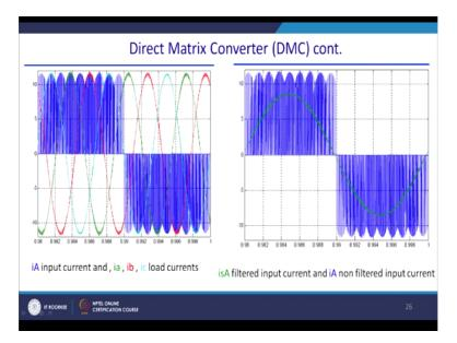
So this is actually a three-phase waveform for input site and ultimately you generate blue one as your output and you are basically now reducing the frequency of the output voltage and you can actually get this is your input and this is your output voltage.
