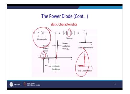
And you know this is the structures, this is a PN junction in between you have extra layer that is you might have seen, this is -drift region, -n layer has been put inside it to give you a reverse voltage blocking capability and this is basically the forward characteristics of the diode, it is same but this voltage may not be actually 0.7, it is generally higher depending on which amount of the blocking capability that diode have.
