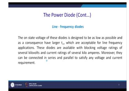
Low frequency diode is normally used for the rectifier operations and we want actually lower conduction loss because it can carry then higher current and drop will be lower but it will have a soft recovery or a slow recovery. So the on state voltage of the diode is designed to be low as possible as a consequence it has larger trr which are acceptable for the line frequency applications in 50 hertz or 60 hertz depending on the countries you are using.
