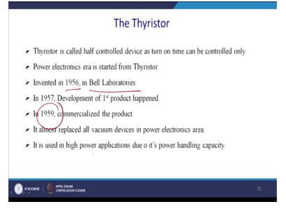
So the thyristors is called half controlled device and as turn on time can be controlled only. So you can control when to turn it on and it has got a forward blocking voltage capability and we can say that power electronics era started with the invention of the thyristor. Thus, we get into the venture into the power electronics when thyristors becomes fully functional and we can play around thyristors in those days.
