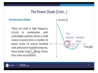
So fast recovery diode actually will go from this point to this point, so basically this is the region you know this is the current, if you integrate over time, this is the charge. Ultimately, your depletion region should hold very less amount of charge that is the only solution to provide a fast recovery and that is used for the high frequency application. So if you integrate over it though this gives you the charge.
