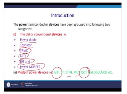
Thereafter, GTO since thyristor does not have a turn off capability, it require an external procedure to turn on that is called commutations and we can turn off a kind of thyristors with negative gate current so that will be GTO that will also be covered. Thereafter, BJT this is also power BJT because in analog electronics we have studied BJT but that power handling capability is quite low in watt.
