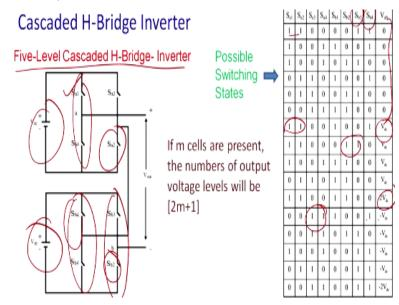
Basically a two independent voltage source if you do not choose the same source an independent voltage source then the residing voltage will shot and you will get 0 voltage and for this reason we have to ensure that these are different. Now these are getting applications for green field solar
