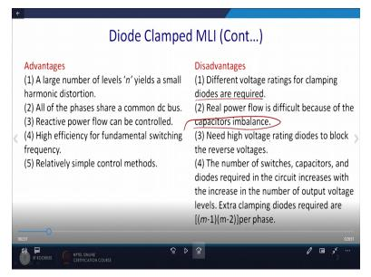
All the phases share that common dc bus. So this is a common for diode clamped multi-level inverter as we will as the capacitor clamped level inverter. Reactive power flow can be controlled high efficiency for the fundamental switching frequency and relative simple control methods.
