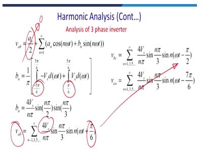
That you know till -5pi/6 to +5pi/6 a voltage actually for the phase A is –VS. Thereafter, till this value, it is positive. So you can calculate and while by integration, the value of BAn will come out to be 4VS/nPi where n can be any integer sin n pi/2sin n pi/3. So this will be the basically the BM. So what should be the value of AB, AB will be essentially you subtract. So you will get 1, 3, 5 0 to infinity 4VS/n pi/sin n pi/3 sin n omega T+pi/6.
