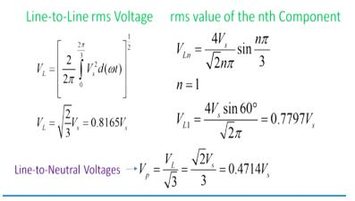
Now harmonic analysis, so what is the amount of the harmonic present into the system. So line to line voltage, RMS value of the component. So VL of course this voltage across the inductor you can integrate over it. So 2/2pi, actually you will know that it will conduct for a period of 2pi/3, so V square S ddt1/2. So this value will be root 2/root 3\*VS that is 0.8165 something like that.
