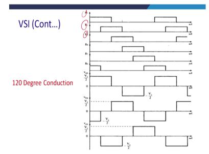
Now let us see that the conductions for 120 degrees, mode of conduction, this is G1, G2, G3, G4 and all the pulses and switches will conduct for the period of 120 degree and then we have phase shifted all these pulses will have a 60 degree phase shifted. G1 and G2 will have 60 degree phase shifted and these are the gate pulses and corresponding switches will be actually T1 or S1 as you have seen.
