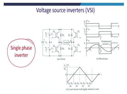
So let us see that this is the simplest form of the inverter. It is in a breach configuration and you can first, we assume that load is highly inductive. So there is no challenge involved if load is resistive. So voltage and current will be in a phase and thus you do not have much problem, but if it is a lagging kind of aspect is there, voltage is lagging, kind is lagging the voltage by 90 degree then you will find that current is at peak when you require to switch it off.
