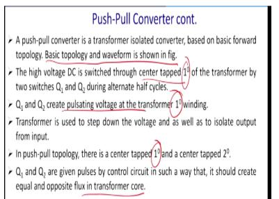
Push Pull converter is isolated transformer isolated converter is a transformer isolated converter based on basic forward converter topology it is been super imposed by the 2 basic topologies of the wave form shown in the figure in previous slides. The high voltage DC is switched on to the centre tapped of primary by a transformer by switch q1 and q2 in an alternate cycle. Q1 and Q2 create pulsating voltage as a transformer winding.
