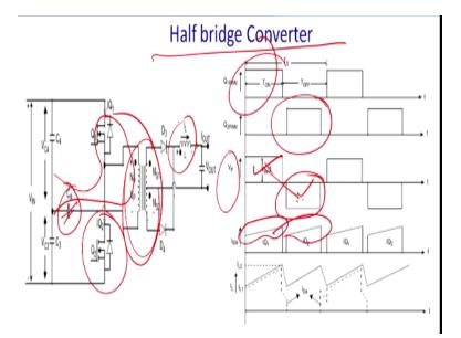
So, instead of actually this push pull converter one of the disadvantage of the push pull converter that it use the central trap transformer and thus it is with required extra winding and it is bulky and costly and there we go for another topology since it uses the 2 switches it is the half bridge converter. Half bridge converter uses 2 switches you have to give a DC blocking capacitor what happens generally this q 1 and q2 may have a small difference of the time period.
