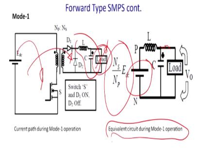
So, see that this is the switch and you have to control this output voltage irrespective of the load. Load may change but output voltage required to be maintained constant so what happen if you couple you know equivalent and this circuit it is been shorted and transformer will transfer power to the primary or secondary and essentially you couple the whole element here and that boils downs to this part of the circuits.
