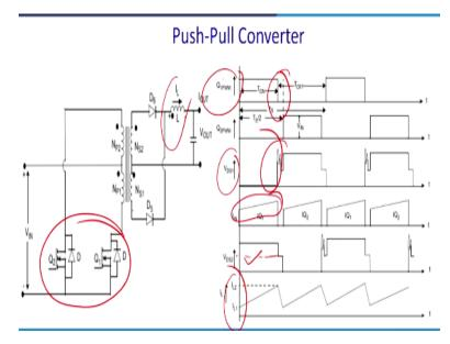
This component count is also increased it has the 2 switches but we will see that what are the actually the voltage is across the switch. And accordingly we will see the devices now you see that these are the pulses of switch 1 this and this is the pulses of switch 2 and that required to be separated by small time duration. And once actually since there is an inductance in the circuit so there would be a spikes.
