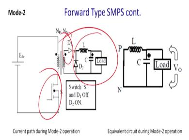
When this switch is off and thus D1 is off ultimately this portion of the circuits plays and it we are assume that D2 is ideal that it can be shorted so you get this part of the circuit to be actually constituted and the filling to the load. So, this is the oscillations of the network.
