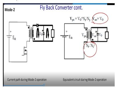
This is a condition of mode 2 when switch is off and but what happened then basically primary voltage will be V0\*Np/NS so this will be the actually the primary voltage. So ultimately there we have a voltage stress across a switch that is proportional to V0 NP/NS.
