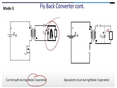
Now current path during this half period so this is a third mode of operation and when actually current has decayed in case of that in case of discontinuous conduction mode and what happened you know actually this capacitors essentially is the feeding this load. So let us analysis this part of the circuit so this will be feeding the load and switch is off because it is in a discontinuous conduction mode.
