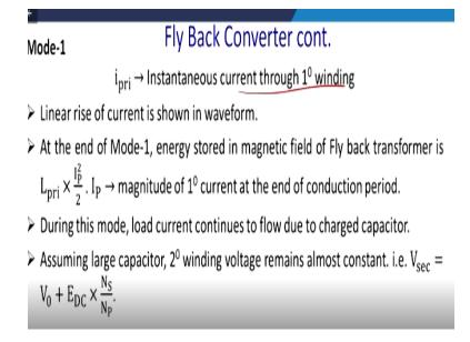
This is primary instantaneous current through the winding 1. Linear rise of that current is shown in the wave form and since L=l d/dt at the end of mode 1 energy stored in the magnetic field of the fly back transformer is L pri Ip square/2\*IP the magnitude of first wining current at the end of the conduction period has been shown. During this mode load current continues to flow due to discharge of the capacitor and assume that this is a continuous conduction mode.
