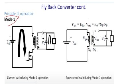
So this is our assumption based on our assumption we are going for this analysis. So mode 1 when switch is on so what happened when switch is on effectively sell he becomes this so current will flow through it and this is NP/NS. So since diode is reverse bias no power flows into a secondary. Since this polarity and due to the dot convention you will have this polarity so this diode will have a reverse biased.
