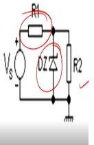
So shunt regulator is essentially who can simplify like this there is a you have studied in the analogue electronics. So that is you got a current control resistance and this a Zener it will have a sharp cut off voltage and you will get a regulated voltage here. So Shunt regulator provides a path for the supply of the voltage but there will be a constant power dissipation across this R1 path supply the voltage to the ground through the variable resistance.
