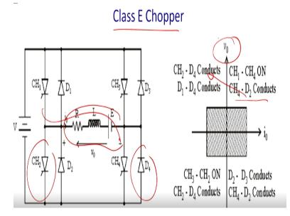
It is actually all the mode of operations for it is possible. So first quadrant mostly so first squadron mostly CH1 and CH2 is on while it is actually current flow in these directions and CH2 and DH2 conducts. So when it is actually regenerative braking then just this will have an interchange this nomenclature will have a inter change that is CH2 n D4 will conduct so CH2 and D4 will conduct and you will get a regenerative braking.
