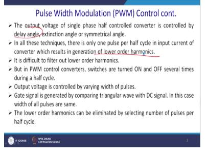
The output voltage of the single phase half controlled PWM converter is controlled by delay angle; this one is a delay angle and extinction angle or a symmetrical angle. All these techniques are only one pulse half cycle in the input current which we have shown in the previous class. Current of the converter which results in generation of the lower order harmonics, so this is one of the difficulty of it.
