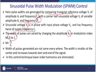
Now, here the pulse rate are generated by as we have discussed here comparing the triangular reference voltage Vr of the amplitude Ar and the frequency as of the supply frequency Fr with the carrier sinusoidal voltage Vc of the variable amplitude Ac of the frequency double frequency oscillation. So you have to rectify it and get it done. The sinusoidal voltage Vc is the phase with the input voltage Vs and has frequency twice of supply frequency Fs.
