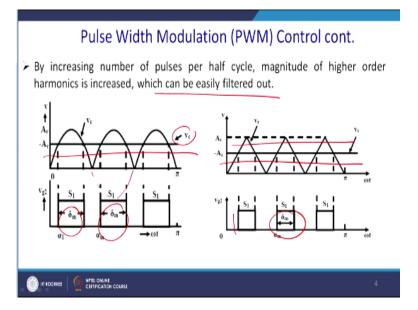
So just see that this is actually the sinusoidal wave form and its replica. So you can change this value Vc and thus you can change the value of Dm. So by increasing the number of pulse per half cycle, magnitude of the higher order harmonics is increasing, which can easily be filtered out.
