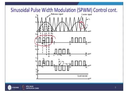
Now we can choose a triangular wave that is quite higher than this supply frequency mostly actually the Vc will be at the supply frequency. So accordingly you have a multiple pulses can be generated and for this reason you will find that actually the width since you are comparing width here it will be more and here width will be narrow. So in that way it will vary. So similarly you can have this kind of variations of the input current.
