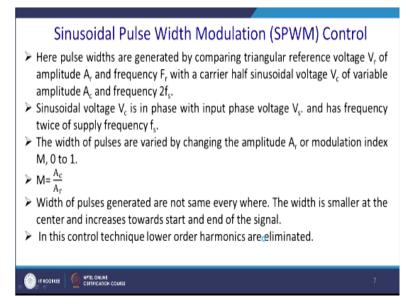
So you require to calculate the value of bm so it is 1/pi 0 to 2pi Is sin omega T so we have a P such pulses in a half cycle so it is 1 to P summation of that if you do that integration you will get basically 2iA where A is the constant output current by Mpi m=1 to P cos in alpha – bm square. So you know you see that you can choose this actually alpha in such a way that value of bm can be made 0, so if you trigger at ones you can actually eliminate only one alpha.
