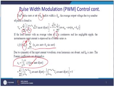
Let us see consider that Mth pulse starts alpha m and with the modulation index delta m with a average output voltage due to P number of pulses is required to be found out. So we can have the summation 1 to P 2/pi alpha m to alpha m+Dm Vm sin omega T you can actually integrate operate so you will root T/pi so you get a summation.
