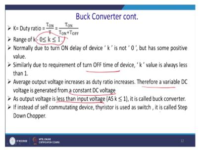
So while K is the Duty ratio that is T ON/T, so you can write in this format also. T ON T ON+ T OFF. So range of the k will vary from 0 to k, 0 to 1 so you can choose any duty cycle for the continuous conduction mode and you will get up actually direction relation between the input and the output voltage. Normally due to ON delay the device k is not equal to 0 and has some positive value because you cannot have 0 turn ON time as well as turn OFF time.
