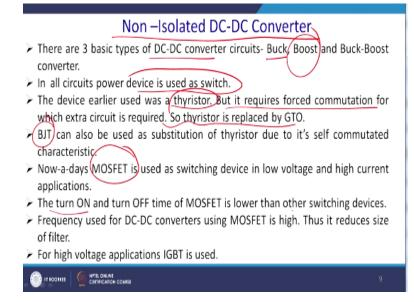
Today we will discuss about the Non-Isolated DC to DC converter. Definitely there is another part of it there is a isolated DC to DC converter. So input and the output stage has got the Galvanic isolation. But SMPS is definitely the DC to DC converter, non-isolated DC to DC converter. So of course depending upon the application.
