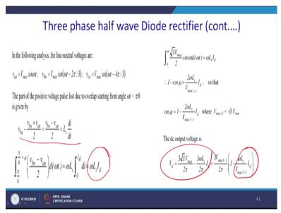
From there we can calculate so you can calculate basically the what should be the value of the Bn and what should be value of the An and thus what we can do, you can calculate the average value of it. So while calculating average value you can find it our; it is almost same 3Vmax/2pi 1- this part is basically coming for the source inductance and so this is actually the integration is pi/6 to pi/6+Mu.
