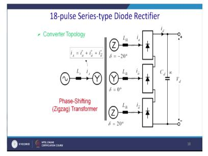
Now let us take the 18-pulse converter. Of course the complexity will increase so we will have one Zigzag transformer. Since we have 18-pulse so it require to a special design. So the phase difference between this transformer require to be actually 20 degree, so that is something a special arrangement, special kind of transformer is required to be built to fit into the system and this kind of transformer is called Zigzag transformer.
