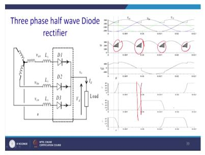
Similarly, same thing can be explored to the three phase half wave diode bridge rectifier. And this is the actually the overlapping time, so this is the actually ia, this is ib and overlapping time is basically the same and due to this overlapping time you will see that fall in voltages.
