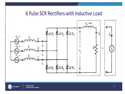
Let us talk about same thing with the controlled rectifier that mean with the converter. Let us go again the 6-pluse and see a rectifier with the inductive load and see that what happens its performance analysis.
