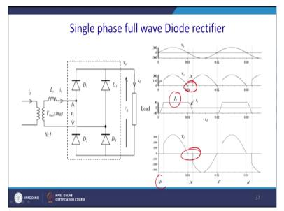
So her also same thing happens, till the point Mu both that actually due to the overlapping angle; here overlapping angle comes into the picture first D1 D4 conducts, D2 conducts and due to that what happen, actually so there will be a overlapping. Once this actually current through this D1 and D4 decades and current through the D2 D3 picks up. And this is the current Id1 across the load and also this is Vi and within this Mu region nothing is takes place.
