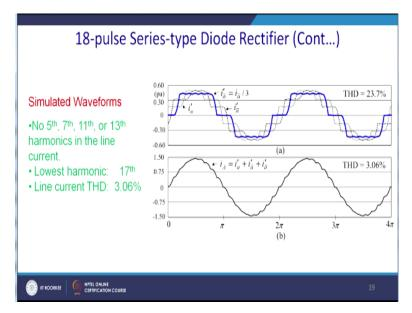
So what happen in case of the 18-pulse converter so if you; there are three current actually as soon into the one by blue other by dot and other by the front line. So these three current consisting of actually the current of the individual rectifier. And if you superimpose these three current ultimately we get the current which is available into the primary and individual THD of this current may be as high as 23%.
