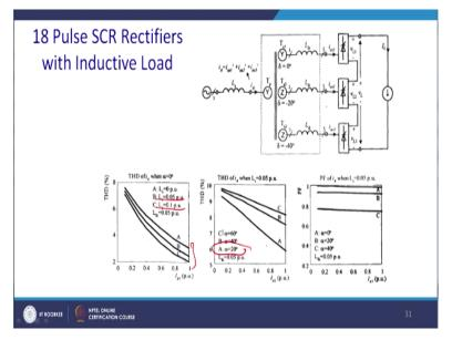
So similarly, what should be the corresponding parameters of 18-pulse converter? So of course they will be phase shifted by 20 degree. And for alpha=0 you can find it out that it actually the THD for the input current will be quite high as 18% but it will come down to around 2%. So and for the little high source inductance it comes down little below similarly, when THD for the different triggered angle will be also actually replicated here.
