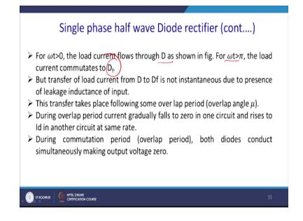
So for a single phase half wave diode rectifier, for omega t > 0, the load current flows the diode when diode D1 as shown in the figure for omega t>pi, the load current commutes to Df. But transfer of load current from D to Df is not instantaneous due to the presence of the inputs of the leakage inductance. This transfer takes place following some overlap period of which is actually marked by the angle Mu.
