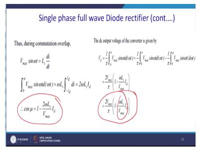
So the same calculation has to be repeated so Vmax sin omega t = Ls di/dt for the source inductance and this value what we have calculated same. So dc output voltage we require to calculate so it is 1/pi 0 to Vmax sin omega t– 1/pi 0 to Mu and ultimately you come across this expression of the output voltage decreased that is basically this part is been the decreased part due to the actually the overlapping angle.
