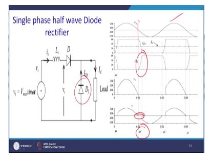
Now let us take a simple example of a source inductance with the free wave diode single phase half wave rectifier. So what happens you know this is a source voltage we have to; this is the current Id because it picks up once this current 0 because of the source inductance it will try to conduct. And you know this will actually fall but it is not instantaneous that the Df will pick up, so there will be time Df will pickup, for this is Df will pickup sometime it will continue to flow.
