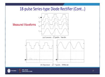
So this the waveform of the 16-pulse converter so; this is actually ia, ia bar delta and this is if you impose this three currents together and this becomes the basically essentially the value of this input current and this is the harmonic spectrum real data and you can sign that actually all the this is the harmonic spectrum of the primary of this 18-pulse converter.
