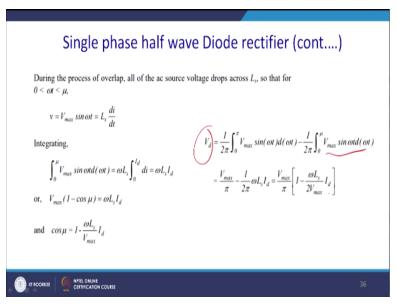
So we can calculate so in a simplest form, so Vm\* sin omega t and it is feeding L di/dt. So while integrating over the time we essentially get the value of the cos Mu and the cos Mu basically called 1-omega Ls or Vmax into the Id. So similarly, we can calculate Vdd and since this zone 0 to Mu it does not get any voltage so output voltage comes down and we require to subtract that voltage.
