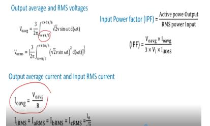
So it is alpha+ pi/6 to alpha +5 pi/6 from there we can calculate the vRMS and IRMS and ultimately from there we can divided it by R to calculate the average current and IRMS you will find that I0/root 3 by simple calculations since it is a square. So similarly we can calculate the input power factor that is V output average/ I output average \*3\*Vrms\*Irms. So let us come to the more practicable solutions of the three phase.
