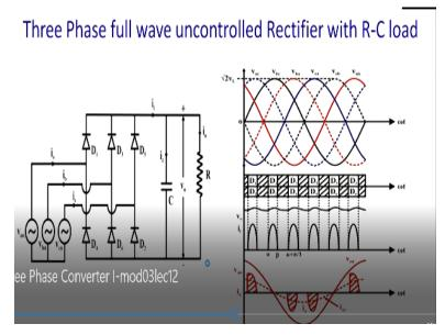
So now let us see that what happen if this actually three phase full wave uncontrolled rectifier fitting in RC load that is quite common you know actually most of the application nowadays are adjustable speed drive. In case of the adjustable speed drive actually you can have a variable kind of load and what happen you know you fit to an inverter to run it in the drives in a different manner.
