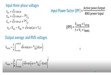
So it does not lead to the saturation on the transformer similarly we required to calculate that actually the Vrms and the average voltages. So students are requested to calculate this value you know actually this is a simple integrations and it is available in normal any textbook.
