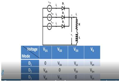
Since actually most of our supply is three phase three wave or four wave system and it makes sense for the high power applications for the dc motor mostly this kind of applications we convert directly three phase to dc. So this is the application part of it so we use this is basically three phase half wave uncontrolled rectifier fitted through the diodes and it is fitting data I assume that RL load.
