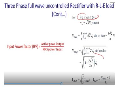
Now few parameters comes into the pictures now for as we start from this actually pi/3 to 2 pi/3 and AC is the amount of the voltage coming into the picture. So output voltage will be given by 3 pi/ 3 to pi 3 VL sin omega t from there we can get this basically the value of the RMS voltage. RMS voltage you can find it out at this 1+3 root 3/2 pi\*VL. So from there of course you know you have a RMS voltage just divide by the you can find it out the current.
