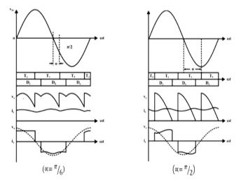
Three Phase full wave half controlled Rectifier (Cont...)
