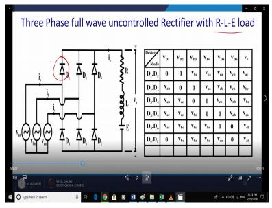
Now, since we are discussed that this mode of the actually configuration is not preferred because it leads to the saturation of the transformer and the rate of the conversion of the power is very low generally use full control devices. The three phase full wave uncontrolled actually rectifier with let us consider the R L E load. Now in this condition one diode from the upper leg and another diode from the lower leg will conduct.
