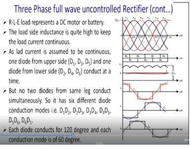
So this is actually a wave form so we consider the RLE load represents the DC mode or the battery and the load side inductance is quite high to keep the load current continuous. So we have a ripple but actually this is a Idc value and the load current assumed to be continuous one diode from the upper side is D1 D3 D5 and another diode from the lower side will conduct at a time. But no two diodes from the same leg will conduct simultaneously
