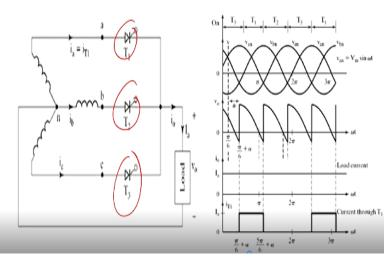
So there is a Thyristor iT1 and there is no difference in between the diode and the Thyristor we required to trigger the forward most forward Thyristor depending on the voltages and automatically other Thyristor will naturally commutate it. Because if this let us say that previously b phase was the most positive and Thyristor T2 was actually conducting the moment actually F has become more positive.
