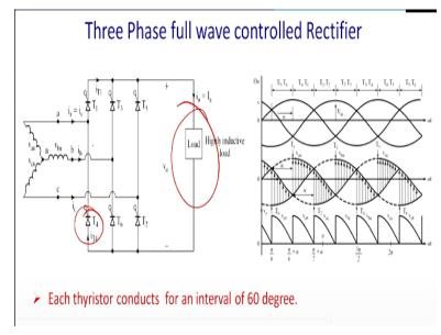
So since it will be conducting and one pair of Thyristor will be conducting for the period of 60 degree phi/3 and 1 thyristor itself will be conducting for the period of 120 degree and what will happen here in this case essentially we will have a same kind of actually nomenclature that is T1 T3 T5 are the upper thyristors and T4 T6 T2 are the lower thyristors. So you trigger the point where phase A and phase C are crossing over.
