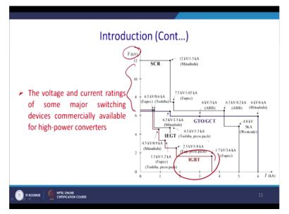
So this is actually the device rating that we can talk about today. You can see that SCR has huge voltage rating and it is available and it can operate actually 12 kV and 1.5 kilo ampere of current. Thus, you multiply this power rating goes as high as actually MVA or mega volt rating. So you can see gradually you know so thereafter but it is a half controlled device, you can turn it on or turn off, has to have a complicated process.
