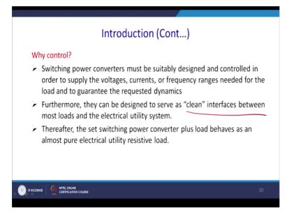
So switching power converter must be suitably designed and controlled in order to supply the required voltage current and other requirement and for this reason we require to be effectively control it and it is a feedback control and different kind of control technique is possible and we will find that actually. They can be design and serve as a clean interface between the load and the electrical utility.
