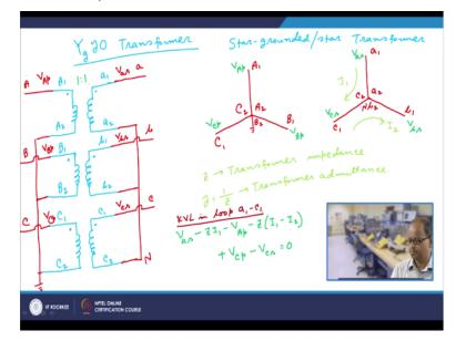
So therefore today what we are going to do is modeling of Ygy transformer, so it is Ygy transformer, so let us say Ygy0 transformer. So that means it is basically star-grounded star transformer and there is no phase difference between the phase A voltage of the primary side and the phase a voltage of the secondary side. So then therefore, we again draw, so we have got as we have done so have got 3 winding, as you have done in the earlier case you are doing exactly the same case.
