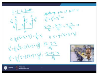
So let us start so fault analysis, so what we are doing is so now we are considering L-L-L fault. So this L-L-L fault is we have a, b, c we have so this is an L-L-L fault please note that so this is Iaf, Ibf, Icf and these are all zf, zf, zf. So let us see that these are all given as zf. So now let us so that this point is N neutral points, so then therefore applying KCL at N, applying KCL at point N that Iaf+Ibf+Icf=0 so we get Va-VN/zf+Vb-VN/vf+Vc-VN/zf=0.
