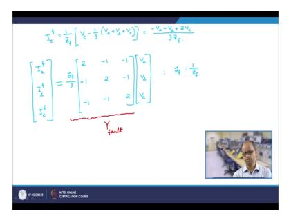
And Icf is 1/zf\*Vc-1/3 Va+Vb+Vc so it is -Va-Vb+2Vc/3zf. So then therefore, if I put all of them in a matrix form, it would be yf/3 2 -1 -1 -1 2 -1 -1 2 Va Vb Vc where yf is=1/zf. So then therefore, this quantity is nothing but Y fault right. So this is Y fault, which is easier. So now let us look at L-L-L-G fault.
