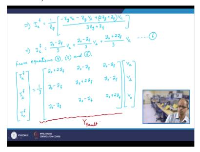
So it would be Icf would be 1/zf-zg Va-zg Vb+2zg+zf Vc/3zg+zf. So in other words Icf is essentially y0-yf/3\*Va+y0-yf/3\*Vb+y0+2yf/3\*Vc. So from equation 4, 5, 6 we can write down, what you can write down, you can Iaf Ibf Icf=1/3 so it is y0+2yf y0-yf y0-yf this is y0-yf y0+2yf y0-yf y0-yf y0-yf y0+2yf and this is into Va Vb Vc. So therefore this is the Y fault matrix.
