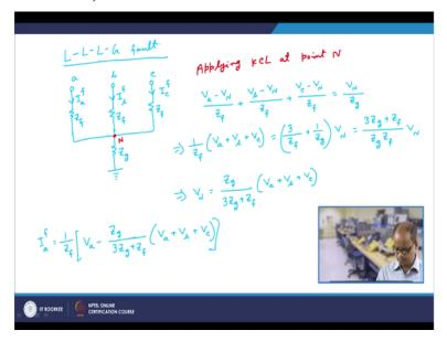
So now we are looking at L-L-L-G fault. So what we have, we have is and then we have so what we will have is so if a, b, c all are zf, zf, zf, zg, Icf, Ibf, Iaf. Again, as usual we take this point to be let us say N, this point is N, so applying KCL at point N, what we can write down, we can write down that Va-VN/zf+Vb-VN/zf+Vc-VN/zf is=VN/zg. So then therefore, we have 1/zf\*Va+Vb+Vc is=3/zf+1/zg\*VN.
