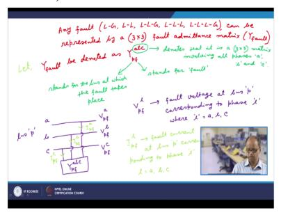
So it means that for any fault either L-G or L-L or L-L-G or L-L-L or L-L-G any fault can be represented by a 3 x 3 fault admittance matrix so this is Y fault. In short, when we would be writing as in Y fault let us denote as Y fault as Y let us say pf abc. So here what does this p stands for, p stands for here essentially let Y fault be denoted as we should write that Y fault be denoted as Ypf abc.
