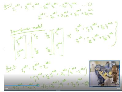
As shown here and we and now we would be now essentially writing the equations for bus 2 bus 3 bus 4 bus 5 and after that you would be writing these equations writing those equations in a matrix form to ultimately form the Y bus matrix. Now for the purpose of writing the equation in at bus 2 and bus 3 let us denote that this bus 2 is denoted as bus m so let us say that bus 2 is bus m and let us say that bus 3 is bus m.
