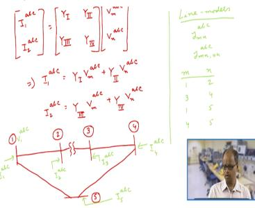
Which is shown here which is basically a fibre system 1 2 3 4 5 and there are basically 4 lines between the buses 1 2 3 4 1 5 and 4 5 and we have also 1 transformer 3 phase transformed between bus 2 and 3 and we are also earlier shown that any 3 phase unbalance transformer having okay any kind of transformer connection can be modelled by this kind of equation I1 abc I2 abc= this y1 y2 y3 y4 \*vm abc and vn abc.
