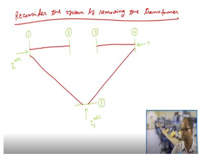
So now we what we will do is not we will reconsider the system. By removing the transformer so if I reconsider the system by removing the transformer then this system looks like this so I have got bus 1 and then bus 2 bus 3 bust 4 and bus 5 so this was bus 1 this was bus 2 bus 3 this is bus 4 this is bus 5 and we have also this lines are connected between bus 1 and 2 between bus 3 and 4 between bus 4 and 5 and between bus 4 and 5.
