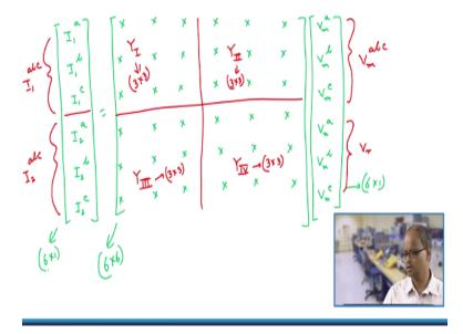
I1a I1b I1c I2a I2bI2c these are 6 current quantities please note that all these currents are complex current so because so this is a 6\*1 and here also V1a V1b V sorry this should be Vn so this should be Vna Vmb and Vmc Vna Vnb Vnc so this is also 6\*1 so now obviously this matrix s would be 6\*6 matrix so now what happens that are depending upon the transformer connection right.
