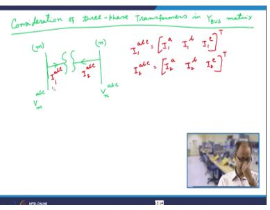
So, the next is consideration of transformer in waivers matrix so the next step is consideration of 3 phase transformer in Y bus matrix so now let us say that we have a bus we have 2 buses. Let us say bus m and n and between please note that this is basically a 3 phase bus. So, then it is voltages again Vm abc and this voltage is Vn abc and between these 2 buses there is one 3 phase transformers connected.
