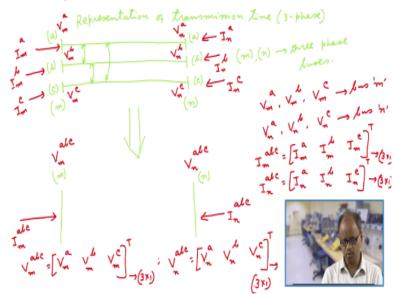
So now we have to now do something like representation of transmission line. So representation of transmission line representation of transmission line. We are actually talking about three phase. Now suppose now here for this representation of a transmission line we do take some particular notation. Now suppose I do have a bus m and bus n this is bus n. Please note that this is bus m and n are 3 phase buses bus m and n are 3 phase buses right.
