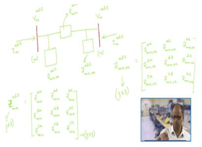
So for the representation of the lines what we do simply write like this. So what we have got is essentially so this voltage is Vmabc this voltage is Vnabc. Current is Imabc this current Inabc this is bus n and this is bus m and the line is represented by a matrix. It is a 3 cross 3 matrix and the half line charging susceptances are also represented by a 3 cross 3 matrix this is also represented by as 3 cross 3 matrix.
