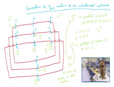
So what we have been discussing is that we have shown a very simple 4 bus network, bus 1, bus 2, bus 3 and bus 4 with this connection and we also noticed that in contrast to the single phase case in the case of a three phase unbalanced system there would be actually 3 N number of injected current as well as 3 N number of voltages. So therefore we should say that there is actually 3 N number of injected current.
