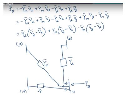
So, Iy-Ym vu+Ym vv -Ydvx+Ydvy so -Ydvx+Ydvyall these are complex. So we Ym vu+Ym vv-Ydvx+Ydvy and we add and subtract Ym vy-Ym vy these are complex. So we take these two terms Yd\*vy-vx +Ym\*vy-vu- Ym so we have taken for this we have taken this term and this term and the last vy -vv. So this term and this term so again we have u v x y. This is Iy this is x this is y this is u this is v Yd\*vy-vx.
