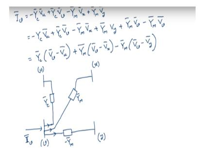
So from this relation Iv we can write down as  $-Yc^*vu+Yc^*vv -Ym vx+Ym vy$  all this are complex we must be careful. So here also we add and subtract from this expression Ym vv and Ym so we add Ym vv and subsequently also subtract Ym vv such that this expression remains the same. So from here we can see that Yc can be written as vv -vu by taking these two terms together +Ym vv – vx by taking this term and this term together.
