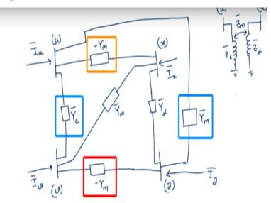
So we again take this as u this is v this is x this is y so -Ym between Y and u so this is -Ym this is Yc u and v is Yc x and y is Yd Y and v is -Ym. And these two need to be done so between u and y there is Ym so to make it between u and y there is 1 Ym and between v and x there is another Ym this we can put here so this is the circuit and as we said Iu Iv Ix Iy so this is the circuit this is the equivalent circuit.
