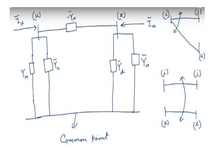
So then what I have got bus u bus and there is a common point. This is the common point this is bus u bus x so between bus u and bus x I still have got -Ym that we cannot have avoid between bus u and v that is the common point there is Yc. Okay and between u and Y also there is another element that is Ym but because v and Y are the same point. So then therefore Ym is also in parallel with Yc.
