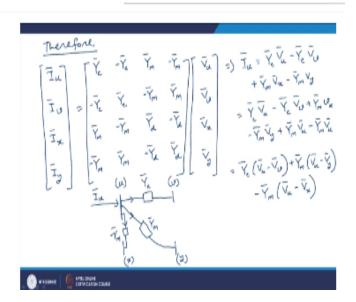
Buses u v x and y between bus u and v there is an element connected having impedance zc between bus x and y there is an element connected having an impedance zd and these 2 elements are also interconnected with each other by an equivalent mutual impedance zn. Iu Iv Ix and Iy those are nothing but the bus injected currents at bus u v x and y respectively. Vu vv vx and vy are nothing but the bus voltages at this buses uv x and y respectively.
