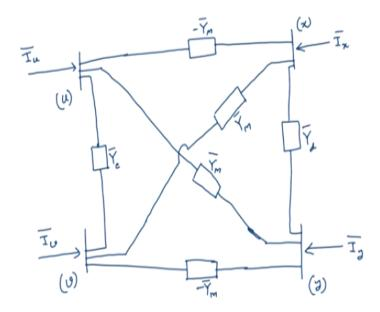
So what do we have is so final equivalent circuit bus u bus v let us make it b1 bus x +bus y so this is bus x this is bus y this is v this is u. Injected current here is Ix injected current here is Iy injected current here it Iu injected current here is Iv? Let us go to the first equivalent circuit first. Okay u and v so between u and v there is an element connected Yc. So between u and v there is an element connected Yc.
