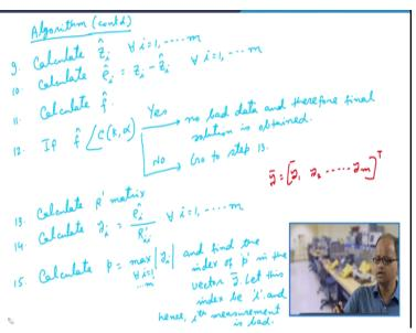
Now, after this also, so algorithm continued, so here also is the solution and from then and we should write here and go back to step 9, so this is actually go to step 9, what do you do in step 9, we calculate, in step 9 calculate zi hat overall i = 1 to m, then step 10 calculate ei hat = zi - zi hat, this is for all i = 1 to m, then we calculate f hat, then what do we do; if f hat is < ck - alpha is no bad data and then therefore, final solution is obtained.
