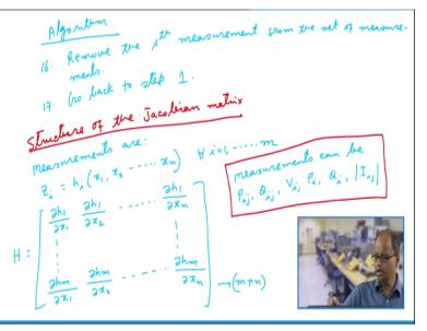
So, then therefore what do we do; remove the lth measurement from the set of measurements, right, go back to step 1, so this is a complete algorithm of the state estimation which includes also the process of bad data deduction now, here, now we have to look into this basically, the structure of this Jacobian matrix, so now let us look at the structure of the Jacobian matrix, so now we are looking at the structure of Jacobian matrix.
