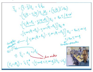
So, then therefore Iij is actually Vi - Vj \* Iij, Vi, Vj are the complex voltages, Vi; so it has got a voltage Vi, this is got a voltage Vj, and we must also write that Vi, Vj complex voltages of bus i and j, and we also should write that Vi = Vi angle theta i and Vji is also be Vj angle theta j and let us say Yij is Yij angle alpha ij, we should not write alpha allowed because we are already utilising alpha, sp something else we should write, should write beta ij.
