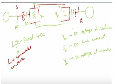
Now in the case of HVDC link what happens? So in the case of HVDC link we all know that basically there is one let us say sending end bus and then there is some converter transformer and there is one converter and then from this converter then we have got this DC line. So this is converter, this is DC line. Then that DC line goes and terminates into another converter.
