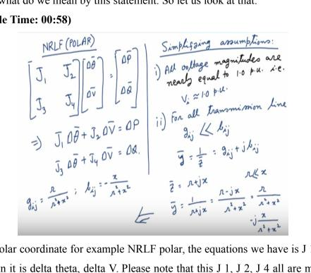
So in the polar coordinate for example NRLF polar, the equations we have is J 1, J 2, J 3, J 4 and then it is delta theta, delta V. Please note that this J 1, J 2, J 4 all are matrices of appropriate dimensions. Then we have delta P, delta Q vector. So then if we do expand this what equations I get? I get J 1 delta theta + J 2 delta V = delta P and we get J 3 delta theta + J 4 delta V = delta Q.
