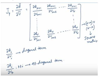
J 4 is del Q/del V. So if I do del Q M + 1/del V M + 1, del Q M + 1/del V M + 2...del V N. And it would go up to last one del Q N/del V M + 1. Then del Q N/del V M + 2... del Q N/del V N. So it would be a (N - M) \* (N - M) matrix. So it is a square matrix. Last 2 were this I must say that this is a rectangular matrix. J 2 is also a rectangular matrix. Okay, so this is a square matrix.
