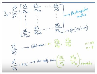
So then therefore del P by del V vector would be and we have also seen that del P the expressions of this the matrices are del P 2/del V + 1, del P 2/del V + 2...del P 2/del V N and then it goes up to then del P N/del V M + 1. Then del P N/del V M + 2. And then last is N. And it would be essentially an (N - 1) \* (N - M) matrix. So then it is a rectangular matrix.
