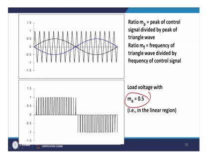
So, this is actually the b a PWM wave form and that will be generating and assuming that actually the value of ma as 0.5. That means it is in a linear region.
