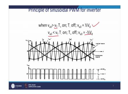
So, let us now see that what is now the, what is the functionality and principle of operation of the inverter? Please go back this circuit. And see that what are the switch has been mentioned, this is a half breast combinations and in a half breast combinations average voltage applied across is BDC by 2. And so this is the upper switch and this is the lower switch.
