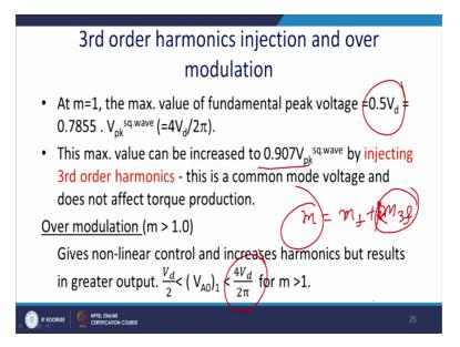
So, what are the advantages of it so at m equal to 1 modulating index equal to 1 so, ongoing part of the saturation. So, the value of the fundamental voltage it is actually 0.5 V d c and that is basically you know 4 by d by 2 pi for the half bridge configuration.
