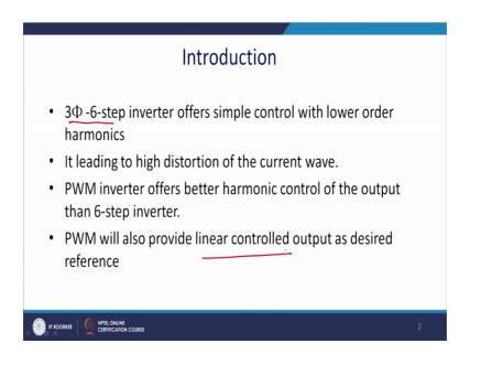
But, and it also contained lower order harmonics that is one of the disadvantage of this kind of converter. And that leads to the higher current distortion. PWM on the other hand PWM inverter on the other hand can actually offer better harmonic better TSD, because here what happen here? It actually voltage harmonic almost remain same, but current harmonic actually been reduced because most of the cases you know facts applications on the drive system.
