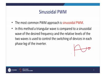
Here, in what happens in this case sin wave that is mostly the control wave or the modulating wave, it will be actually compared with the triangle wave and we accordingly actually reference will be generated we can see the next slide.
