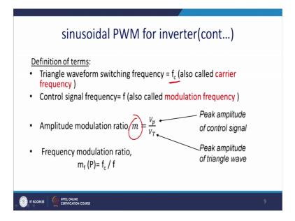
We, refer actually the triangular wire frequency a triangular wave frequency or the carrier frequency and it will be referred as a f c and same way the control frequency will
