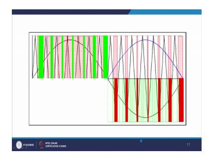
So, ultimately this will be subtracted from it that this is basically A voltage and this is which is a B voltage and ultimately this will get subtracted. And so, you get actually the resultant wave form something like this.
