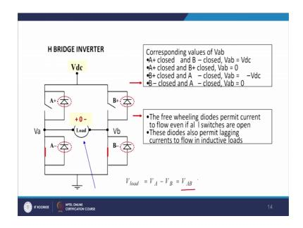
In this case actually load voltage again will be V A be and we have already discussed how the what is the principle operation? And this is a principle operation when actually we see that when diode conducts? When switches conduct and other thing.
