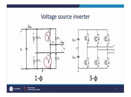
And, we take a simple breast wire simple breast topology of the 2 level inverter subsequently classes we should discuss about the PWM applicable for the 3 level inverter and it is applications.
