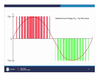
And, what is the advantage of it? Advantage of it that actually it is instantaneous voltage error is half. Since, let us consider that this is actually the sin wave where actually volt area curve is as matched. And so, for this you can find that voltage error here actually will be actually only half of the error voltage that compared to the bipolar.
