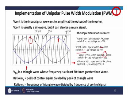
Now, let us come to this actually unipolar PWM operation. In this case actually you require a V sin omega T and the minus V sin omega T and you require actually this inverted signal also. So, that is basically you require little bit more complex circuit, but it
