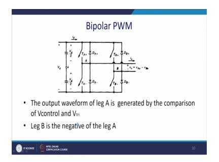
Now, again let us go back to the same circuit and we shall discuss about a bipolar PWM and it is a simplest PWM of itself. And the output voltage of the leg a is generally a compulsion between precontrol and the V T or V tri and leg B is nega leg B is a negative of the leg a and this is actually the bridge configuration.
