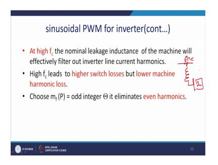
High frequency normal leakage inductance of the machine will effectively filtered out and thus inverted current or in case of the STATCOM was in case of the facts an application. Generally, we connect the pole of the inverter with we will connect pole of the inverter that is this point is called point of common coupling with an inductor with the inverter.
