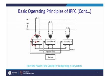
Now, this is a line. So, this is converter 1. And all generally have a common dc link. And this is connected via transformer, because of the rating, because it is connected in the high voltage line. So, power electronic device cannot directly sustain that rating for this will be required to have a step down transformer.
