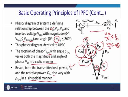
So, let us discuss about the actually the first line of IPFC. So, this is the one line diagram of IPFC with single a, and this is a phasor of the IPFC. So, you can see that actually before compensation, this was the V s 1, this magnitude was V s 1. And effectively that angle was delta 1.
