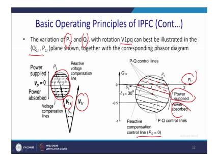
So, the variation of the P 1, and Q 1, with rotation of the V 1 q can be best illustrated in sending-end power that is P 1 r, and P q r, shown in the plane, together that correspond to the phasor diagram. See that this is the V s 1, and this is actually V r 1, and this is circle is basic essential is a sphere of influence. And the compensating voltage line are this dotted quads. And the reactive power compensation lines are basically the board lines.
