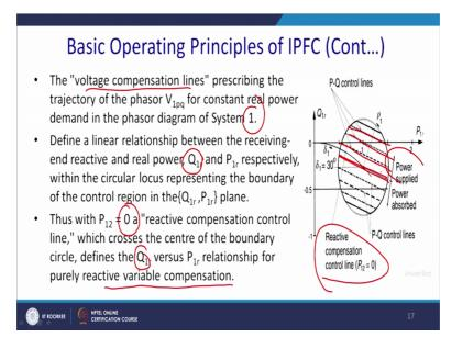
Thus, voltage compensation line prescribing the trajectory for the phasor p 1 q for the constant real power demands in the phasor diagram of system 1. So, this is the power supplied above it above the diameter, and this is a power absorbed, and this is the P-Q line, these are the constant P-Q line with if it operates in this P-Q line, you know this is a constant P-Q line.
