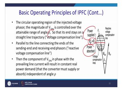
So, operate the circular operating region that is a circle of interference. Region of the injected voltage of the phasor, at and the magnitude V p 1, V 1 p q is controlled over the attainable angle rho. So, that its end stays on the straight line trajectory, that mean you have to operate in this line.
