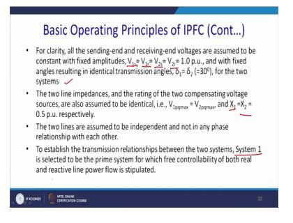
Now, for clarity, let us let us take all those condition in advance. All the sending-end and the receiving-end voltage, assumed to be constant with the fix amplitude, that mean V s 1, V r 1, V s 2, V r 2 all are at one per unit at its base values. With the fix angle, resulting the identical transmission angles, let us say delta equal to delta 1 equal to delta 2 equal to let us say to 30 degree or 45 degree, for the two machine model.
