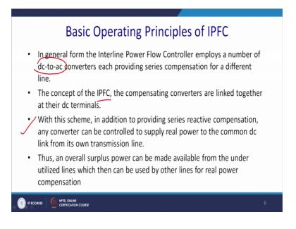
So, in general form of intermit and power flow controller implies is the same number of dc-to-ac converters, each providing series compensation of different lines. The concept of IPSC IPFC, the composite converter is linked together by the terminal. And the dc links are common, will come to this actually the picture in next slides.
