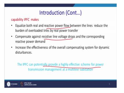
So, what we can state what is actually its capability. IPFC makes equalized both real and reactive power flow between the line, and reduces the burden of the overloaded line for real power transfer. It is a typical case in railways, where may be the one line is heavily loaded, because of the there has a the trucks is running in a particular line, and other lines are not so much overloaded So, IPFC finds huge application in this kind of system.
