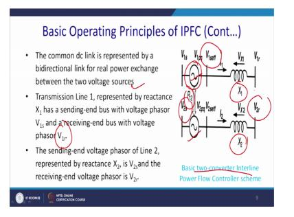
So, let us take us these pictures. So, this is a basic two-converter intermit and powerful line conditioner scheme. So, this is basically your V P 1, so actually it will inject it will inject the voltage same way, the series compensation of p q. And effectively these voltage become V 1 effective, and thus you can same power.
