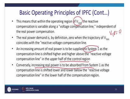
So, this means that within the operating region V 1 p q, the reactive compensation is variable along a voltage compensation line, independent of the real power compensation. The real power demand is, by definition zero, when trajectory of V 1 p q coincide with the reactive voltage compensation line. So, we when you are actually V p 1 essentially is 0, then your real power compensation is 0.
