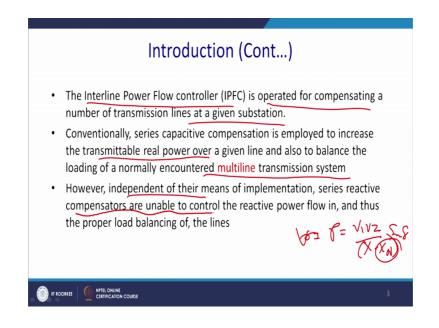
Now, we shall discuss, now the Interline Power Flow Controller. And we see the, limitation of the normal shunt compensations, series compensation, mostly series compensations, because power flow can be handled at by the series compensation. And will find the limitations of it.
