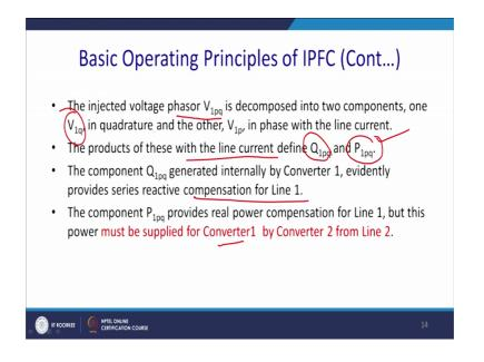
The voltage injection of the phasor V 1 p q, it decompose into the two components, one definitely V 1 q that is a reactive component of it, then quadratures, and other V 1 p, in phase with the line current. The product of these with the line current defined, Q 1 p q, similarly with a in phase component with I give you P 1 p q.
