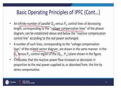
So, from the discussions, we can say that an infinite number of parallel lines, parallel P parallel Q 1 r verses P 1 r lines of decreasing length corresponding to the voltage composition line as you go up for the phasor diagram, can be established. So, what happened, you know this length decreases as we go up the compensation increases. Similarly, also you decrease.
