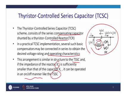
This thyristors controlled series capacitor so, it is a improved version of the previous version of TSSC, the thyristors controlled series capacitor TCSC scheme consists of the series compensating capacitor shunted by the thyristor controlled reactor. So, you will have a inductor here, in practical TCSC implementation several such basic [com/compensator] compensator may be connected in series to obtain the desired voltage rating and the operating characteristics.
