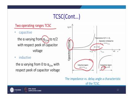
You can change with the alpha and here is the region where you can change alpha angle actually triggering angle. So, it is equal to 0 to minimum alpha, similarly the C limit will change, alpha C limit will change accordingly. So, when it will be capacitive, this is a two mode of operation in TCSC the alpha varying from I C alpha minimum or limit to pi by 2 with respect to the peak of the capacitor voltage.
