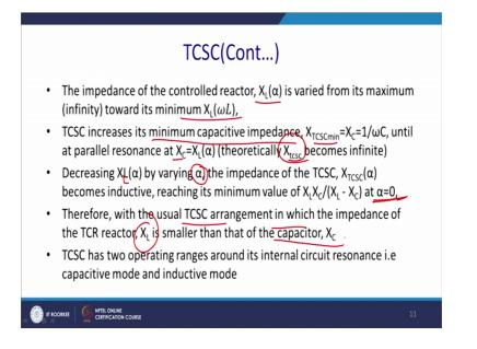
The impedance of the controlled reactor X L alpha is varied from its maximum to the infinity towards minimum X L. The TCSC increases its minimum capacitive impedance that is TCSC minimum equal to X C equal to 1 by omega C until the parallel resonance at X C equal to X L alpha and theoretically it becomes infinite, so thus it can offer a huge impedance.
