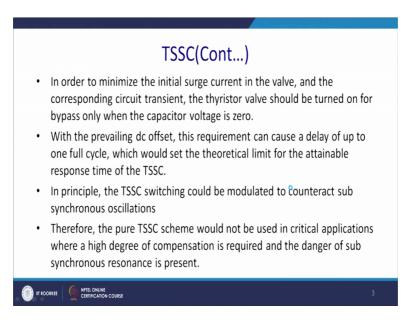
So, I am the control intern and control technique, in order to minimize the initials surge current in the valve and the corresponding circuit transient; the thyristor valve should be turn on or bypass only when capacitor voltage is received.
