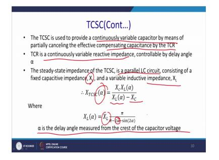
The TCSC is use to provide a continuously variable capacitor by means of partially cancelling the effective compensating capacitance by TCR. TCR is a continuously variable reactive impedance controlled by the delay angle alpha, this steady state impedance of the TCSC is a parallel LC circuits consisting of a fixed impedance X C and the variable impedance X L.
