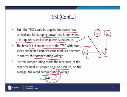
But this TSSC could be applied for the power flow control and for damping power oscillation where required speed response is moderate. So, this is the where it can find its application, you say this is the V Cmax the maximum V C can be applied and this is the I V characteristics. And accordingly this value can be changed, this is I max and this is I min within the range you can operate you can choose any value of the admittance.
