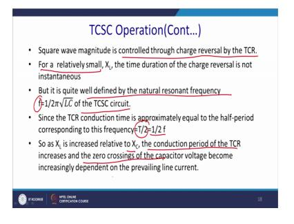
So, what we can say more about the TCSC. So, square wave magnitude is controlled through the charge reversal by TCR. For relatively small X L the time duration of a charge reversal is not instantaneous, it will take some time. But, it is quite well defined by the natural frequency of oscillation where f is basically 1 by under root of omega C; So, omega C under root of l c for the TCSC circuit.
