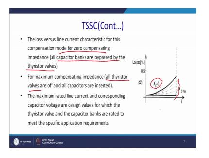
The loss versus line current characteristics for this compensation mode for the 0 compensating impedance, all capacitor banks are bypassed by the thyristor valve. For maximum compensating impedance all thyristor valves are off, all the capacitors are inserted. So, this is the losses, you know this is for X C equal to 0 you will have maximum losses, gradually over it is bypassed so, switching losses will come down gradually.
