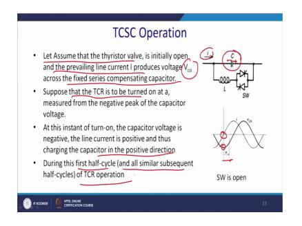
Let us assume that the thyristor valve is initially open. So, all the current was passing through the capacitor and thus what happen, and the prevailing line current produces the voltage V C0 across the fixed compensated capacitor, so across this device.
