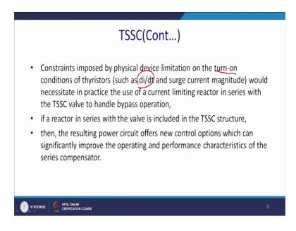
Such as di dt protections of the surge current magnitude would necessitate in practice to use a current limiting reactor, for this is it is not only capacitor, there will be a current limiting device that will give you di dt protection, in series with the TCSC valve to handle the bypass operation. Because if the capacitor discharged with the thyristors, high current will flow through the thyristor with high di dt that may damage thyristor.
