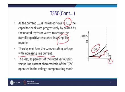
So, what happens then as a results when I min is increased towards I max so, losses will increase definitely. The capacitor banks are progressively by passed by the by the, by the thyristor valve to reduce the overall capacitance and the in a spike like manner. So, you had a, for this is in you have this kind of spikes in admittance, thereby, you maintain the compensation voltage with increase in current limit.
