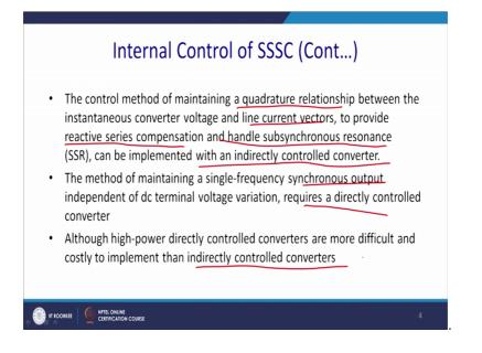
The control method of maintaining a quadrature relationship between the instantaneous converter voltage and a line current vector, to provide the reactive series compensation and handle the sub synchronous resonance or S S R can be implemented with indirectly controlled converter. So, you just control the phase angle rest it will take care of by the deceiver's voltage.
