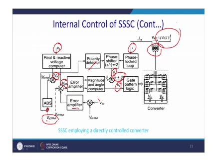
So, this is the internal control of directly controlled circuit and we have to actually have both phi plus theta and the V q. So, you have to fed both this logic to the gate pattern. So, let us see that what are the difference from it is internal from it is indirect control technique. The real magnitude of the computer actually will compute the V q and you have a V q reference, and you have V small q capital Q reference and from there actually you subtract you get V small q capital Q.
