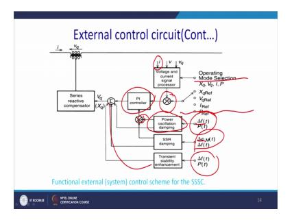
So, this is the overall structures. So, this is basically for the transient stability this is for the sub synchronous oscillation this is for the power frequency oscillation damping. So, this is the mode of some operant d of different mode of operation. So, this is the overall external control circuit for the any kind of series compensator.
