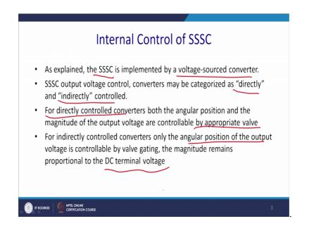
Now, how S S S C can be controlled? Please note that this control technique, which we are discussing, it is more or less combine for all the series type compensator. As explained, triple S C is implemented by a voltage sourced converter.
