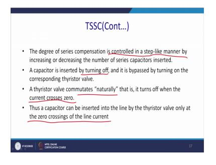
So, degree of the series compensation is controlled like a step manner by increasing or the decreasing the number of the series capacitor inserted into the line.
