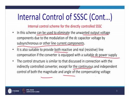
So, from this discussions of the internal control technique we can conclude this scheme can be used to eliminate the unwanted voltage component due to the modulation of the d c capacitor voltage by sub synchronous or other line component, that is one of the biggest problem in power system sub synchronous oscillation that can be camped out by the triple S C.
