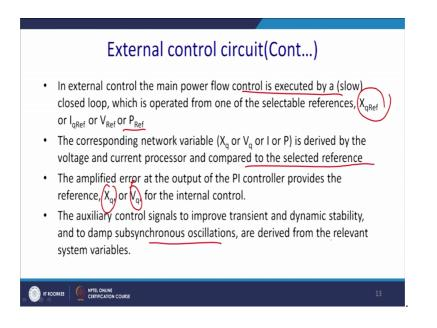
So, in in internal control the main power flow control is executed by a slow closed loop, which is operated from one of the selective reference that is X q Ref I q Ref V Ref or P Ref whatever will be, the corresponding to the network available the X q V q I or P is derived by the voltage current processes and compared to selected reference.
