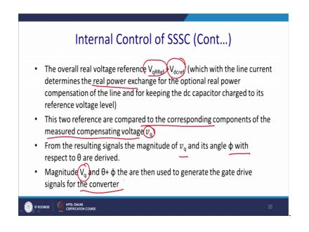
So, overall voltage reference for this direct control will be actually V q R ref plus V d c ref. Which with the line current determines the real power exchange, for the proportional real power compensation of the line and for keeping the d c capacitor charged to the some reference voltage, this is the requirement.
