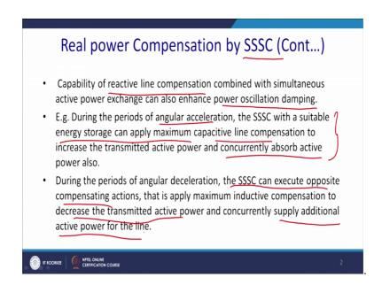
The capability of the reactive line compensations combined with simultaneous the active power exchange can also enhance the power oscillation damping. So, triple S C can provide the active damping. For example, during the period of the angular acceleration the triple S C with a suitable energy storage can supply, the maximum capacitive of the line compensation to increase the transmitted power and concurrently absorb the active powers.
