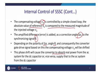
Then, the compensating voltage in the v q is controlled by the simply a closed loop, control the absolute value of the reference V q is compared with the measured magnitude of the injected V q. And, thus we have a error and we fed this error to the P I controller. The amplified difference or the error is added and as a correction angle alpha.
