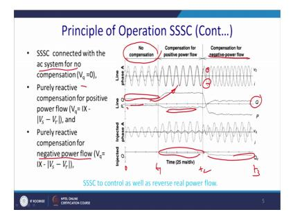
So, that is also possible please see the compensation. So, let us try to understand this graph this is actually without compensation, while voltage in current assumed to be in a phase.
