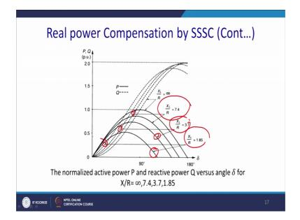
And, thus what happens you can see that line changes. So, this is the uncompensated line where actually X by 1 ratio X 1 by R ratio is and on certain 0.4, but when this ratio changes in a compensated line then, what then this is the case for uncompensated line having X by 1 ratio equal to 3 by 7. Similarly this is the ratio uncompensated line for X by 1 ratio equal to 1.8 5.
