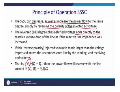
The SSSC can decrease this is a one of the best features of it. As well as increase the power flow in same degree by simply reversing the polarity of the injecting AC voltage. So, it can inject plus V q or it can inject minus V q if plus V q inject increases the voltage capability, you can reduce the capability of the line by injecting minus V q.
