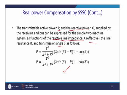
The transmittable reactive power P, and the reactive power Q, supplied by the receiving end bus can be expressed for the simple 2 machine system, as a function of the reactive line impedance effective.
