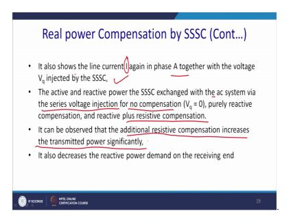
Moreover, it also shows the line current I again in phase a together with the voltage V q injected by S S S C. The active and the reactive power in the SSSC exchanged with the a c system via series voltage injection for no compensation when V q is 0, purely reactive compensation and reactive plus resistive compensation can be also done here.
