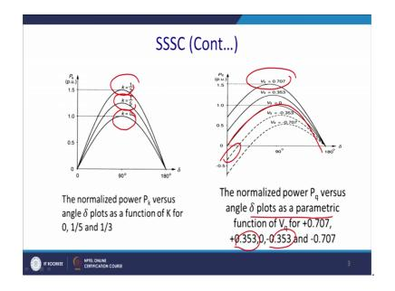
Where k equal to 1 by 5 is a ratio of is a ratio of V by V q and this is one third you can see that at even at one third voltage and 90 degree power handling capability increases to 50 percent.
