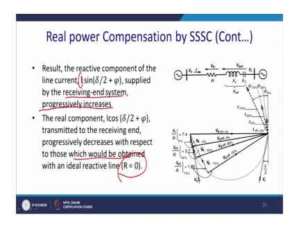
Now, the result of this reacting compensation of the line current sin I sin delta by 2 plus phi supplied by the receiving end system progressively increases, that is the one of the disadvantage. So, so the real component that is I cos delta by 2 plus phi transmitted to the receiving end progressively decreases with respect to those would have been obtained in the ideal reactance line when R equal to 0.
