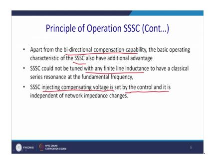
SSSC should not be tuned to any finite line inductance to have a classical series resonance at the fundamental frequency. So, never resonance will occur and high current will flow. This one of the disadvantage of this small system, SSSC injecting compensating voltage is set to keep by keep the control and it is independent of the network impedance changes.
