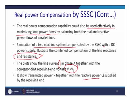
Now, with this observation what we can conclude. The real power compensation capability could also be used effectively in minimizing the loop power flow by balancing both the real and the reactive power flow in the power parallel lines.
