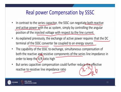
In contrast to the series capacitor triple S C can negotiate both we have assume that actually V q is perpendicular to the I, that is thus current for this is then it is only compensating the reactive power, but we can have a real power compensation. SSSC can negotiate both reactive and the active power with the SSSC system.
