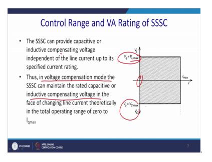
So, the control range of the S S S C. So, ultimately what we can see that. So, you can make V q minus and plus. So, it can go either direction, but current has to be here in uni direction. So, this is the this will operate in first and the fourth quadrant of the I V characteristics. So, SSSC can provide the capacitor and the inductive compensation compensating voltage, independent of the line current up to it is specific current rating as chosen by the device rating.
