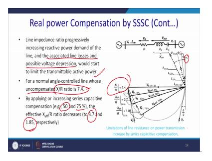
So, voltage sec and other for normal range of control the line whose uncompensated X by R ratio is chosen to be 7.4 that is what I am saying that in previous slide the this ratio is around 7. And, now let us understand this actually the facer as well as the circuit. By applying or increasing the series capacitive impedance let us say 50 percent or 75 percent
