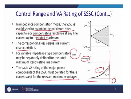
The impedance compensation mode, the SSSC established to maintain the maximum rated capacitive or compensating reactance at any line current up to it is rated voltage up to the rated maximum voltage. Thus what happen the corresponding loss versus line current characteristic is shown here? For this reason this is the I q max and ultimately this is I and this is the loss and this is the current rating of the devices and thus what happen, that is actually will change accordingly.
