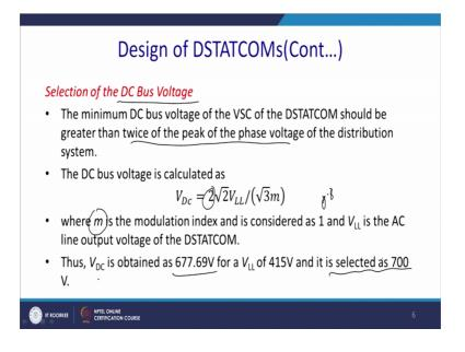
The minimum DC bus voltage of the VSC of the DSTATCOM should be greater than the peak of the phase voltage of the distribution system. The DC bus voltage is calculated as 2 into under root of root 2V by L by root 3m, where modula m is the modulation index and generally it is restricted to 0.8, please mind it.
