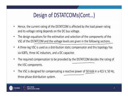
Now, hence, this current rating of the DSTATCOM is affected by the load power rating and the voltage rating depending on the DC bus voltage. The design equation of the estimation and the selection of the component of the VSC of the DSTATCOM and the voltage level are will be discussed in this session.
