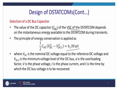
Now, we will talk about the selections of the DC bus capacitor the value of the DC bus capacitor C DC of the VSC of the STATCOM depend on the instantaneous energy available to the STATCOM during the transients. The principle of the energy conversion starts you know half CB square.
