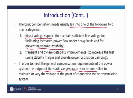
So, the basic compensation needs usually into the following two categories, one the voltage support, direct voltage support to maintain sufficient line voltage facilitating the increase in the power flow under heavy load and for preventing voltage instability. This is may be the purpose another is the transient stability the transient and dynamic stability improvement to increase the first swing stability margin and provide damping to the power oscillation.
