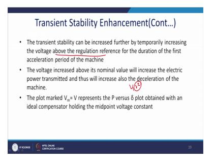
Because you know you have V 1 V 2 if V 2 is increasing. So, power handling capability increases and thus increases also the deceleration of the machine. The plot marked V m equal to V, I shall come now represent the P verses delta power obtained with the ideal compensator holding midpoint voltage constant. So, see that this is the case. So, this is the area and this is the case with the STATCOM and this is the case with the SVC.
