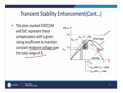
So, this is the SVC and this is basically the STATCOM. So, the plot marks STATCOM and SVC, this compensator with the given rating insufficient to maintain the constant
