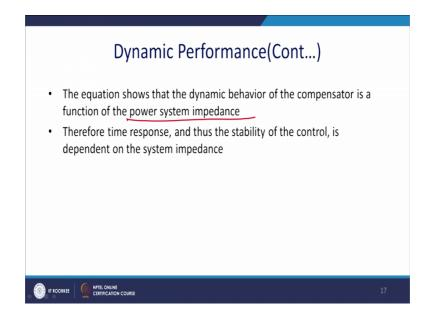
So, SVC basically changes the power system impedance, therefore time response and thus the stability of the control is depend on the system impedance. So, this is something we require to keep in mind. Now transient stability with this SVC; this transient stability indicates the capability of the power system to recover from the major disturbance.
