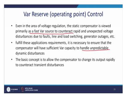
To fulfill this application requirement it is necessary, to ensure that the compensator will have sufficient var capability to handle the unpredictable dynamic disturbances. The basic conserve is to allow the compensator to change this output rapidly to encounter this transient disturbance.
