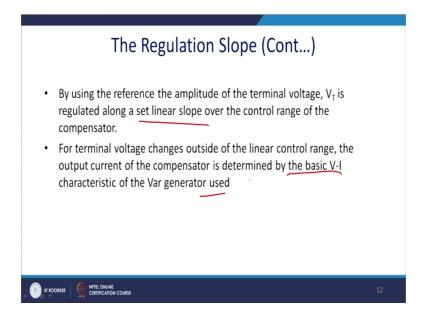
For terminal voltage range outside the linear control range the output current of the compensator is defined by the basic V I characteristic of the Var generator let us see this curve and that will explain the case.
