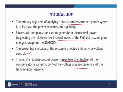
Now, as we know that primary objective of applying the static compensator in a power system is to increase the power transmission capability. This is the basic principle of putting a FACTS devices. Since static compensator cannot generate or absorb real power we have to neglect the switching losses of the SVC, and we should now presently eliminate the idea of putting active component or the storage component with in a STATCOM.
