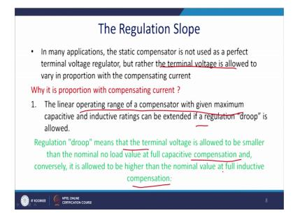
But whether terminal voltage is allowed to vary proportional to the compensating current most of the cases why it is proportional to the compensating current? We know that actually reactive power handling capability varies with the qs in case of the SVC. The linear operating in range of the compensator with the given maximum capacitor and the inducting current can be extended if the regulation droop is allowed.
