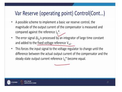
The error signal V Q is then processed by the integrator of the large time constant and added to the fixed value of the voltage reference what happen then? This forces the input signal of the voltage to regulate to change until the difference between the actual output current and the compensator, and the steady state output current reference become equal. So, this is a way to achieve it.
