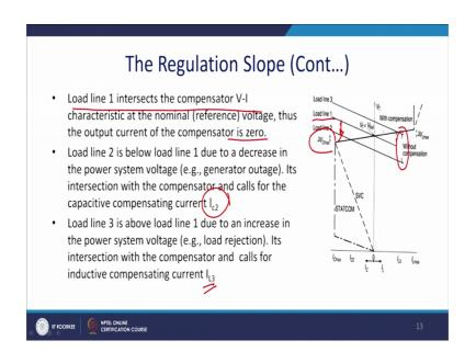
Let us consider that the load line 1 intersects the V I curve. So, this is the load line 1 and this is the load line 1 and the characteristics of the nominal reference voltage and thus what happen? The output current of the compensator is 0 and this is the actually the load line 2. Load line 2 is a below the load line 1 due to decrease in the power system voltage
