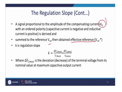
The proportional a signal proportional to the amplitude of the compensating current kIQ with an order of the polarity; capacitive current is negative and the inductive current is positive is derived. Summed to the reference V ref then obtained effective V reference then the V reference will change dynamically as it will be required by the I.
