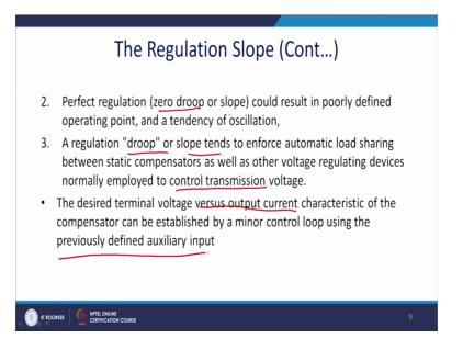
So, that is something we require to prevent the regulation droop or the slope tend to ensure. Automatic load shading between static var compensator as well as the voltage regulating device normally employed to employed to control the transmission voltage. The desired terminal voltage verses the output current characteristics of the compensator can be established by a minor control loop using actually as you have shown a previously defined auxiliary input.
