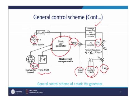
So, this is a general control scheme of SVC what happen you have a prime mover that generates a voltage. So, with an angle V and with voltage V amplitude V and the and the angle delta. So, this is the network and here you put a static var generator, essentially it does not have any power to compensate the real power. So, P is 0 this is the convector converter based and it may be a actually TCSC or TCR. So, what you how you will control it? So, essentially you will measure the voltage.
