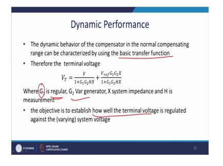
The dynamic behavior of the compensator in a normal compensating range can be characterized by using a basic transfer function and therefore, the terminal voltage V T is V 1 plus G 1 G 2 HX plus V ref G 1 G 2 X 1 plus G 1 G 2 HX am coming to it. So, where G 1 is a regulator, G 2 is a var generator and X is a system impedance and H is the actually the transfer function of the measuring devices. The object is to establish how well terminal voltage is regulated against the varying system voltage.
