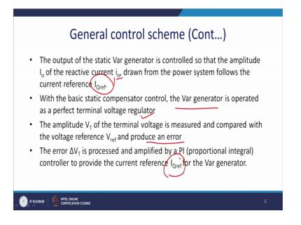
The output of the static Var generator is controlled so, that the amplitude i 0 of reactive current is drawn from the power system and system the reference current IQ ref with the basic compensator control the var generator is operated, at a perfect terminal voltage regulator.
