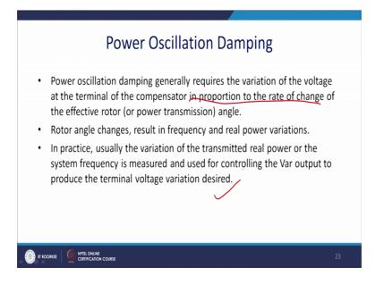
Power oscillation damping we have discussed several time, damping is generally requires the variation of the voltage and the terminal of the compensator in proportional to the rate of change of the effective rotor power angle.
