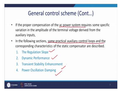
If the proper compensation of the reactive power system require some specific variation of the amplitude of the terminal voltage and that is varied for the auxiliary inputs sometimes it may sac may occur or something. So, there may be the disturbance due to that then we actually work on the auxiliary input.
