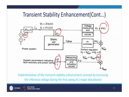
So, power system with fault so, del V has been increased. So, this is basically the change of frequency change of voltage. So, ultimately it will be actually sinking the current i 0 and we have for this reason since it is a del V has been increased.
