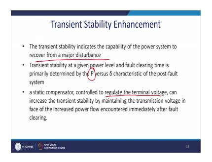
Transient stability at a given power level or the fault clearing time is primarily determined by the power it is actually handling at the moment and the torque angle delta and the post fault system condition. The static compensator controlled to regulate the terminal voltage we have seen that can increase the transient stability by maintaining the transmission line voltage, in the phase of the increased power flow countered immediately after the faults shearing.
