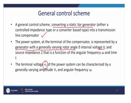
So, this is the one of the desired feature of SVC in general the control scheme converting static var compensator, either to a controlled impedance or a converter type into a transmission line compensator. The power system at the terminal of the compensator is represented by the generator with a generally a varying angle varying rotor angle with the internal voltage V.
