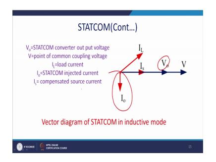
So, STATCOM converter output voltage is V 0 and the system voltage is V and I L is a load current which is leading, and thus STATCOM current will be lagging and it can make the current unity power factor.
