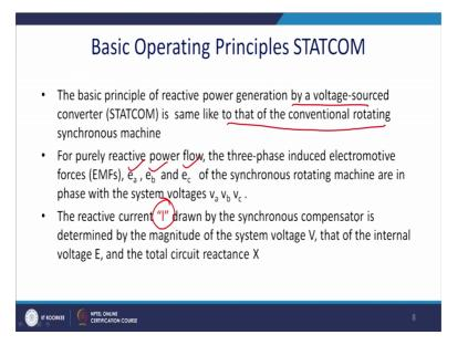
It is there is no difference in it actually, but is a static solution and it is a dynamic solution rotary solution. The purely reactive power flow the 3 phase induced electromagnetic forces e a e b e c of the synchronous rotating machines are in a phase with the system of V a V b V c.
