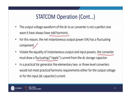
And so, the output voltage wave form of the DC and the AC power is not perfect sine wave and it had always have a odd harmonic, depending on the symmetry we can we can actually eliminate the even harmonic, but odd harmonic will be present. And for this reason the instantaneous output power has a fluctuating component.
