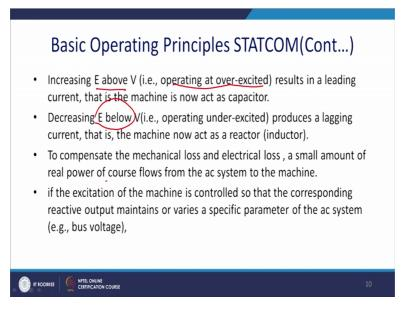
Increasing E above V the operate it is in a over-excited state. Thus result in leading current and that is the machine now acts as a synchronous condenser or a capacitor. Decreasing the value of the E below V the operating as under excited, producing the lagging current and that is a machine acts as an inductor or the reactor.
