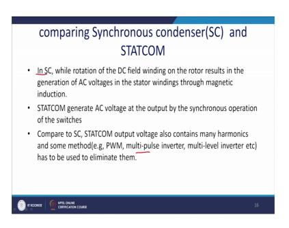
So, thus what we can say? So, what is the difference of the synchronous condenser and the statics and the STATCOM. Synchronous condenser generally have a huge amount of energy requirement in SC the while rotating the DC field winding of the rotor results in the generating the AC voltage in the stator winding through the magnetic induction.
