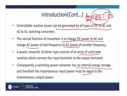
Now, how it works? It controllable reactive power can be generated by all type of AC and DC switching converters. Please understand that what essentially it do we know that it we you we know that, you have you may have a AC system may be it is a PMSM. Thereafter you have an inverter or converter that will convert the DC, thereafter you can convert into the AC.
