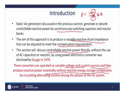
Now, static Var generation discussed in the previous sections S V C, generates or absorb controllable reactive power by synchronously switching the capacitor at the reactor banks.
