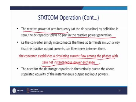
Moreover, reactive power at 0 frequency by definition the reactive power at 0 frequency at that capacitor by definition is 0. The DC capacitor plays no part in fitting the reactive power generation please note that. So, DC capacitor and nothing to do with the reactive power generation. That mean the converter simply interconnect this 3 terminal in a such a way that produces the reactive power. In such a way the reactive power and the voltage and current has to be made at 90 degree phase shift.
