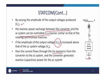
Now, by varying the amplitude of the output voltage produced that will be V 0 when please remember that it is a PWM converter. So, you are switching generally and in may be a multilevel inverter most of the cases. The reactive power changes between the converter and the system can be controlled in a manner similar to that of the rotatary synchronous machine.
