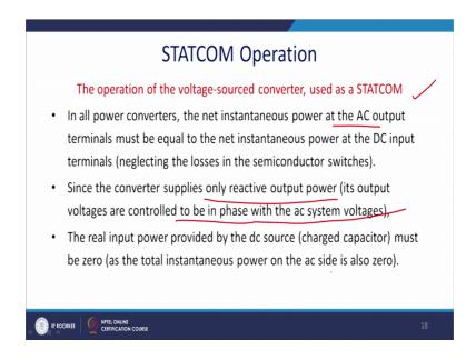
So, for this it is mentioned that operation the voltage source converter at STATCOM. The in all the power converter the instantaneous power at AC output terminal must be equal to the net instantaneous power at the DC output terminal, neglecting the switching losses and other losses neglecting the losses of the semiconductor switches also the hysteresis and (Refer Time: 24:35) losses of the coupled inductor and also those things.
