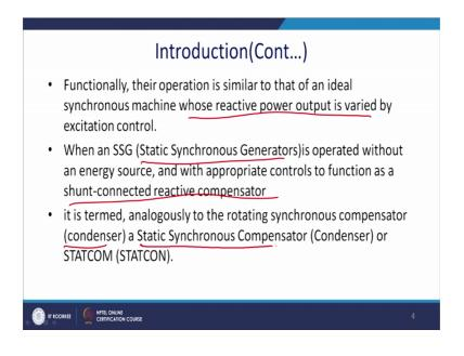
And functionally this operation is similar to the, to an ideal synchronous machine over excited synchronous generator if it is compensating the Var, whose reactive power output is varied by changing the field excitation. Essentially, you have a static solutions what you generally had the rotational solution?
