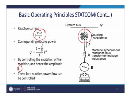
And, thus corresponding to the so, corresponding reactive power will be given by 1 minus E by V by X into V square. By controlling the excitation of the machine hence the amplitude of the E can be controlled and thus therefore, reactive power flow can be controlled.
