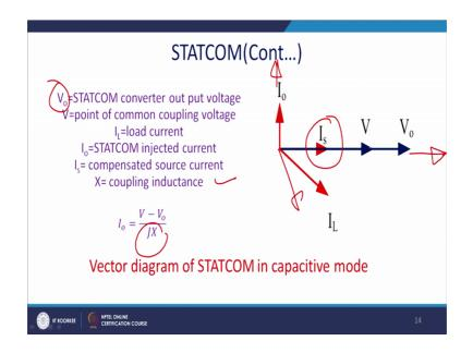
So, what happen here let us see? Let us consider that the output voltage of the STATCOM is V 0 and V the point of the common coupling voltage. What is point of common coupling? This point generally we say that P C C or this point.
