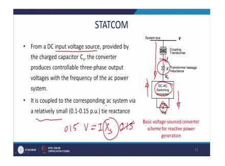
Now, what is STATCOM the principle operation will be same, but here you will have DC to AC switching. So, here also have a actually AC to DC switching we will have a both generally it will in this direction. So, these devices will acts as a converter. So, it will convert and DC energy it will convert to the DC voltage and in this direction it will generate AC.
