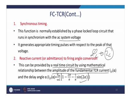
The function is normally is to establish by a phase locked loop circuit, that runs in a synchronism with the ac system, ultimately this is a PLL. It generates the appropriate
