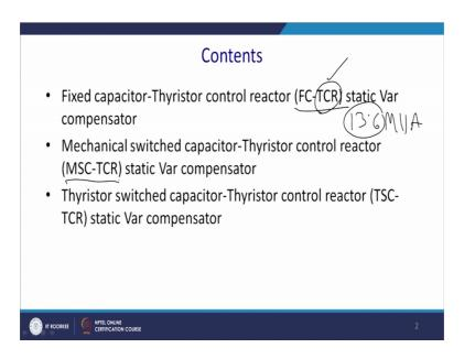
That is fixed capacitor thyristor control reactor. So, where actually the capacitor is fixed with it and thus it gives a kind of compensations and with there actually you got a TCR that will introduce the actually negative var, and in that actually you can have a variable compensator is something like that you require to have a 13.6 positive MVR.
