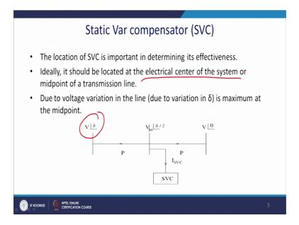
So, this is our convention one line diagram, where actually the sending end voltage is V delta and these are midpoint shunt compensation is put it here.
