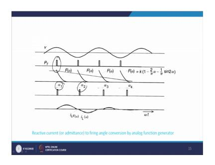
So, this is the voltage and this is the pulse synchronizer, that will come from the PLL and thus this is the amount of the reactive power compensation you require. So, what happen thus you have to change the value of the alpha 1, alpha 2 and so on in some cycles. So, gradually alpha 1 and alpha 2 will change and gradually the current through this inductor will change like this. So, this is the way of implementing this fixed capacitor TCR.
