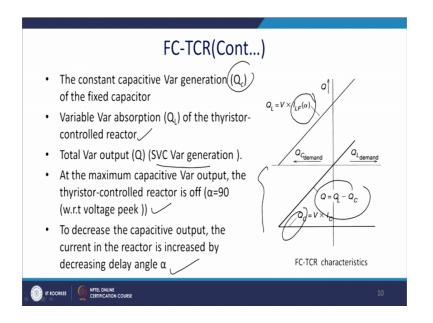
The constant capacitor var generated Q c of the fixed capacitor the variable absorption Q L of the thyristor controlled reactor.
