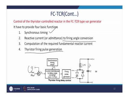
So, how you will generate the control circuit so, first of all we have a four blocks one is synchronous timing. So, that will get from the PLL thereafter reactive current and the current or the admittance for the firing angle conversion, computations of the required fundamental reactor current, thyristor firing generation.
