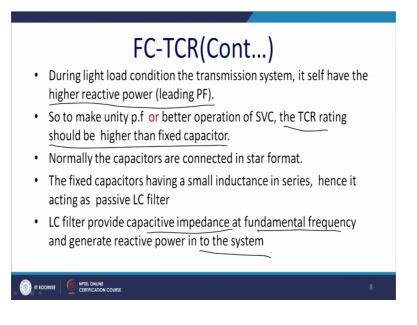
So, there is a problem, you know during the light load condition of the transmission system itself has a higher reactive power or the leading power factor.
