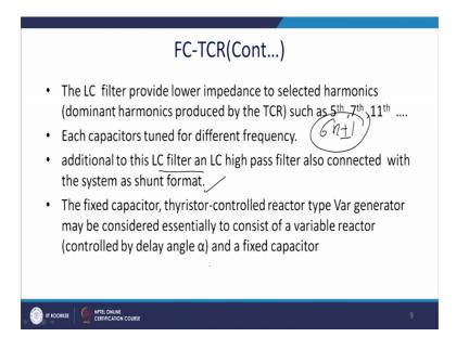
Each capacitor is tuned for the different frequency. Additional to the LC filter an LC high pass filter is also connected with the system as shunt format. The fixed capacitor thyristor controlled reactive reactor type power compensator may be considered essentially to consist of a variable reactor controlled by a delay angle and the fixed capacitor.
