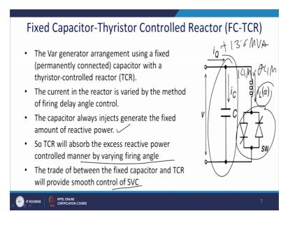
This is basically a fixed capacitor configuration, you have a capacitor that is fixed to the line and ultimately whatever the value of the inductor is required you get it here.
