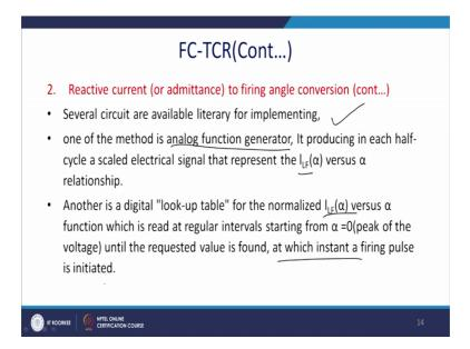
Now, reactive current to the firing angle conversion. Now this is actually we have if you refer to the book you know actually the several circuits. Several circuits are available for the implementation one of the method is for is basically the analog function generator, it will be producing the half cycle scaled electrical signal represent set by the IF alpha and ultimately you can calculate the alpha.
