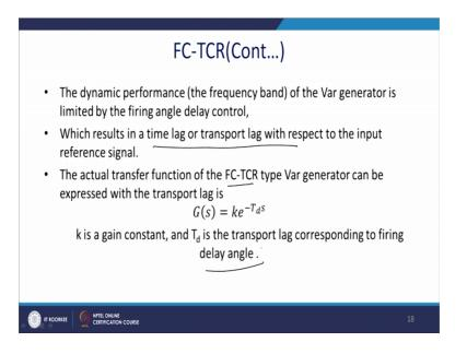
So, what happen here the dynamic performance of the a performance, the frequency band of the var generation is limited by the firing angle delay control. So, it will take a delay because once you have calculated because you are allowed to trigger thyristors after certain interval of time. So, what is in thus there will be a delay in compensation. So, it is a time delay system, which results a time lag or the transportation lag with respect to the input signal reference.
