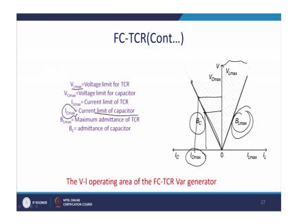
Now, this is the graph this is the fixed graph for this admittance since it is a shunt compensation. So, ultimately this is the I max and this is the BL max, please note that actually voltage (Refer Time: 17:40) of for the capacity compensation. So, for this is you cannot use actually the total rating, but generally voltage sacks for inductive compensation.
