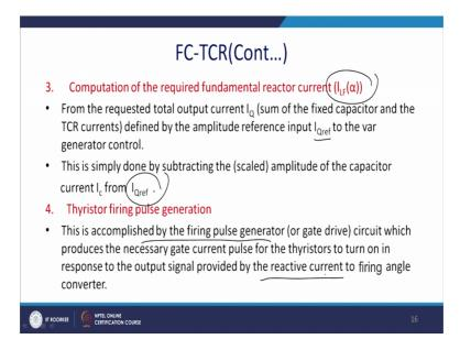
Computations of the required fundamental reactor of IFL alpha; From the requests the total output current Q the sum of the capacitor and the TCR current defined by the
