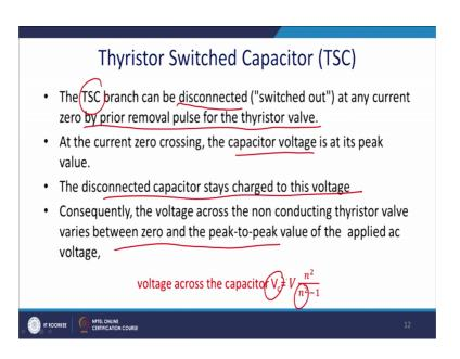
So, the TCSC branch can be disconnected or switched out at any current any current 0 by priorly removing the pulses of the Thyristor valve, this is 1 of the biggest advantage let us understand what does it set.
