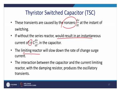
So, considering those thing we require to see few aspects, this transients are caused by nonzero d v d t, you can understand that nonzero d v d t at the instant of the switching. If voltage or current either it is 0 there is no problem. If without series reactor would results the instantaneous current value that is i value should be equal to i equal to C d v d t of the capacitor and to limit this current the limiting what does it do this limiting reactor actually limits this current.
