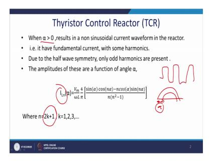
So, this is alpha, so you will have a displacement power factor when alpha that is what it is. So, when alpha is more than 0, so it is a non sinusoidal. And we can do the furrier series analysis current wave form in the reactor the fundamental current will be contaminated with the presence of the harmonics.
