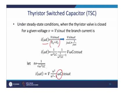
So, ultimately you get the current equal to V n square n minus 1 omega C that is where nothing but x c into  $\cos omega t$ , where m is given by the resonance frequency that is omega square into L c.
