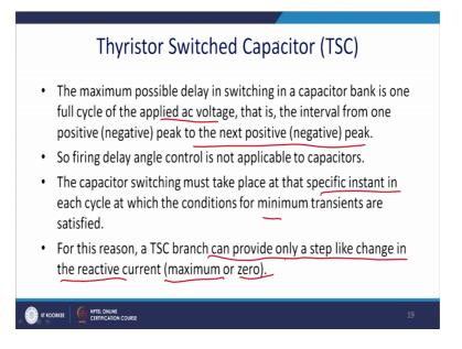
Thyristor switch capacitor the maximum possible delay in switching in the capacitor bank is one of the full cycle is applied to the ac voltage that is the interval of 1 positive or the negative peak to the next negative peak. So, around in case of the 50 s cycle it should be around the 10 millisecond. For firing delay control this not applicable to the capacitor.
