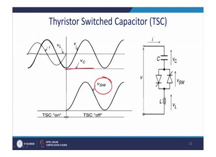
So, this is the current where current is almost lying by 90 degree and this small value is the inductor voltage and what happen here this is the supply voltage and here you have put it off. So, capacitor will maintain this voltage and thus switch will be subjected to this oscillation and we will never stress off actually of the TCSC of this voltage value equal to V. If value of n that is quite logical will be very high, so n square minus 1 is almost equal to n.
