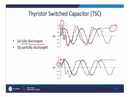
So, what happen? So this is the vc and this value is vi and once is partially fully discharged it has to built some voltage from 0 and thus high current will flow, so the capacitor and current will have a this kind of profile and it will be stabilized after sub cycle. And similarly assuming that this partially discharge and it is voltage is half of the supply voltage and then also you will have a peaky current.
