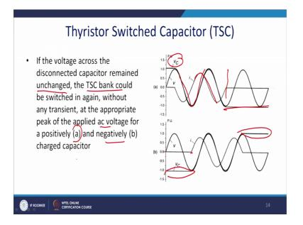
Now, let us consider the case why it was off and this is the voltage VC and it was holding that big value of the voltage and it is on thus voltage will be of the VC will be swinging like this, with the supply voltage and current will have current will be actually will have a showing by 90 degree phase shifted all of a sudden here you put this Thyristor of you have not cleared.
