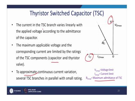
So, now let us see the Thyristor the current in the TCSC branch varies linearly with the applied voltage according to the admittance and it does not have a much problem with the harmonic also. Maximum applied voltage is corresponding to the current are limited by the rating of the TCSC components capacitor and the Thyristors valve.
