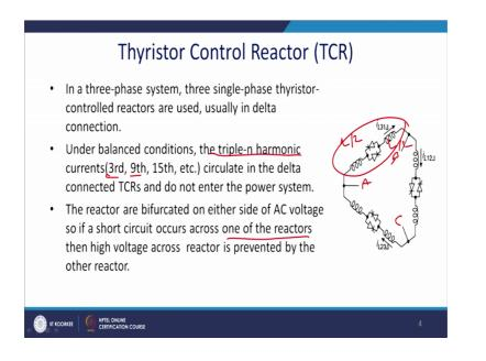
So, we require suppress the third harmonic that is our main concerned in case of the TCR. So, 3 phase system we can put it into the delta, so this is the delta configuration A B and C and this is a delta configuration, if the 3 phase system 3 single phase Thyristor
