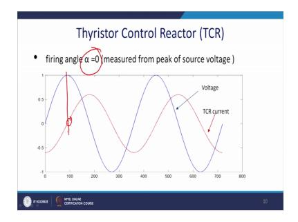
So, what happen here this is the voltage curve for firing angle equal to alpha equal to 0 degree, and this will be the current it will be almost touching the 0 because, but since there is a no pure inductance. So, it will be actually [FL] it is almost yes it is that 90 degree. So, this will be the current so, the TSR TCR at 90 at alpha equal to 0. So, how it will change for different values of alpha?
