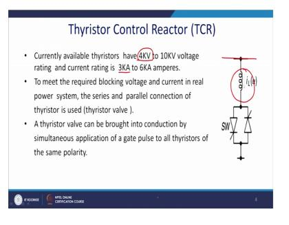
So, generally it is connected in it is a shunt device. So, ultimately you can control the current depending on the switching angle of this thyristors. And generally thyristors are available with a quite high rating and of four point of 4 KV or 10KV most of the cases you know actually there is a factor of safety, for 6.6KV 10KV voltage rating or thyristor is chosen, and of the current rating of 3 kilo ampere or 10 kilo ampere.
