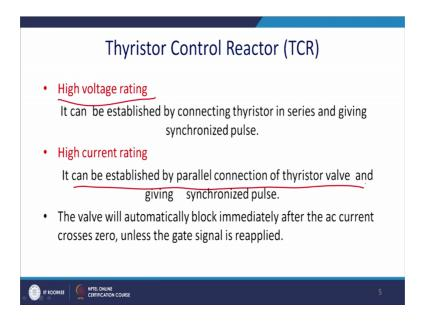
Now, let us talk about thyristor control reactor. So, it can what is a advantage of it? Advantage of it that it has very high voltage ratings since it is a made of thyristors, it can block very high voltage. So, it can be established by connecting thyristors in series and giving synchronization of the pulses. So, that it can turn off and turn on and so, this can be operated for a very high value of the voltage voltage blocking capability.
