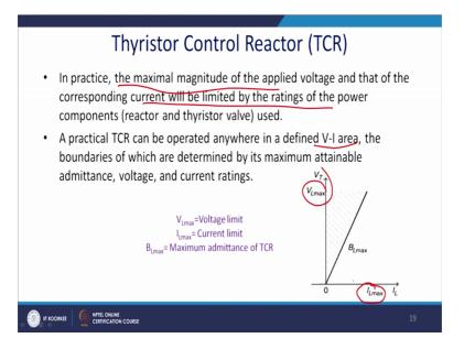
So, what is a thyristor control react? So, in practice what happen? The maximum maximal magnitude of the applied voltage and this corresponding current is limited by the power handling capability of the devices, that is what it is written current will be limited by the rating of the components, that is a thyristor valve in practical TCR can be operated anywhere in defined v a line.
