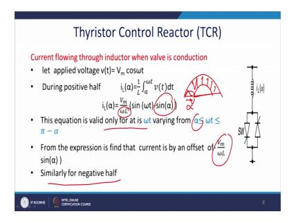
So, we can calculate that what is a value of L here. Since v t is equal to V m cos omega t and during positive wave cycle. So, you are varying i L which is a function of the delay angle will be 1 by L alpha to omega t ultimately this become V m by omega L that is nothing, but x l that is a impedance of this line into sin omega t minus sin alpha.
