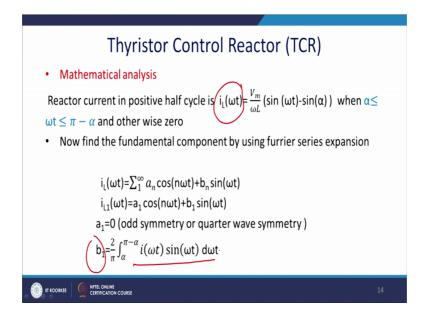
The reactive current let us consider the positive half cycle, that is given by i L omega t is V m by omega L sin omega t minus sin alpha, where alpha is alpha is less than omega t and greater than omega omega t and less than actually pi minus alpha otherwise omega t's value will be equal to 0.
