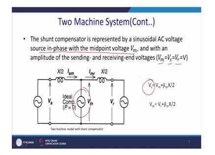
So, shunt compensation represented by the sinusoidal AC voltage and the source in the mid source in-phase with the midpoint V m, and with the amplitude of sending and the receiving end voltage V m equal to V s equal to V r equal to V.
