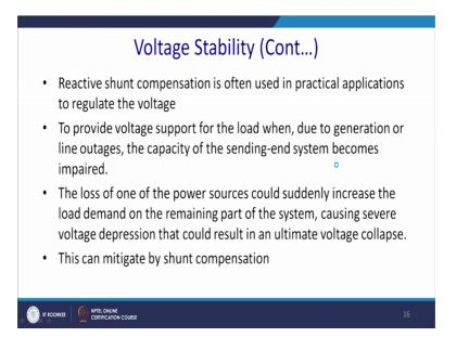
Reactive shunt compensation often used for the practical application to regulate voltage. To provide voltage support for the load and due to the generation of the line outage, the capacity of the sending and system becomes impaired.
