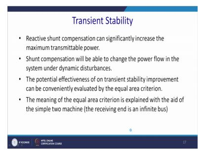
Reactive shunt compensation can significantly increase the transferable power in the line. So, shunt compensation will able to change the power flow in the system under dynamic disturbances. If there is a slight increase in the into the power demand, then it can increase the power handling capability and it can actually bring down this perturbation into the steady state limit.
