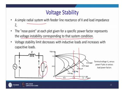
Shunt reactive compensation can effectively increase the voltage stability limit by supplying reactive power to the load and regulating the terminal voltage.
