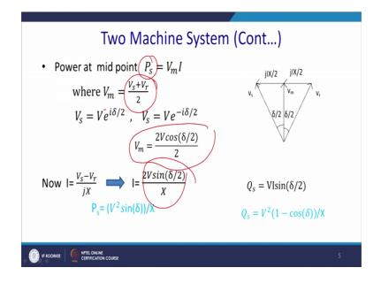
Now, let us see that at the midpoint the power available it P m V equal is P s should be equal to the sending and power that is P m into V I, where V m should be actually instantaneously, it should be V s plus V r by 2. And we have assume that you know V s equal to minus sorry there will be minus delta by 2. So, similarly we can find that this value V m is 2 V cos delta by 2 by 2. Again I flowing this point to this point is V s minus V r by j X.
