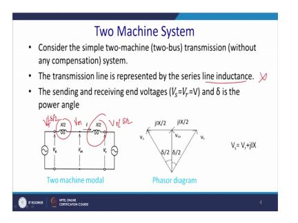
Now, consider the two machine system. So, consider the two machine system and overall transmission line had impedance X. So, which has been spitted in between X 1 and X 2 and this point the voltage is assumed to be actually assumed to be V m and we assume
