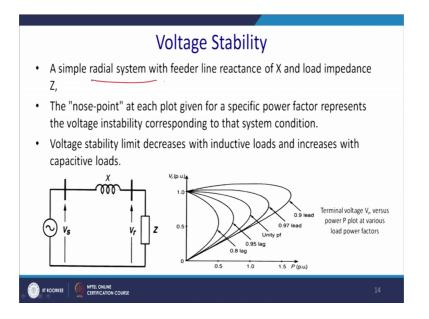
Now, let us see the how a shunt device can stabilise the voltage. So, let us consider a linear network a simple radial system feeder reactance X. The "nose-point" of the each plot is given a power factor; power factor represented by the voltage instability corresponding to that system condition. And voltage stability limit decreases with the inductive loads and increases with a capacitive load.
