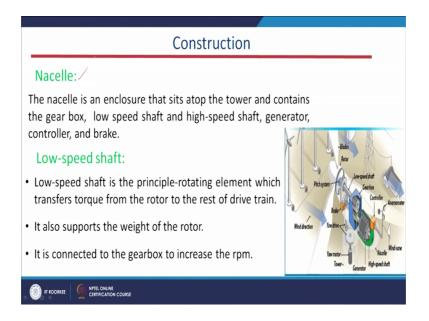
Now, coming to the nacelle this nacelle means it consist of the first one it contains the gear box, will come to function of the gear box, and next one is the low speed shaft and the third one is the high speed shaft generator, controller and the brake.
