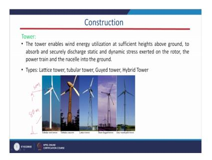
The towel is also important here, if you could see different type of towers we have demonstrated like tabular steel tower, we have tubular, concrete, lattice three legged and different types of tower and for aesthetic look good look and, we are planning also different other types of tower so, also in research in construction.
