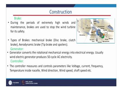
The braking system is a always desirable in every system because, it is a safety consent of the wind system. What is the function of this brake system? Basically during the very stormy condition and, extremely high wind flow. So, we have to basically brake the system operation. So, in that case the braking system is the system which controls or which brakes, the operation of the system. It stopped the wind turbine for its safety that is what the brake system does.
