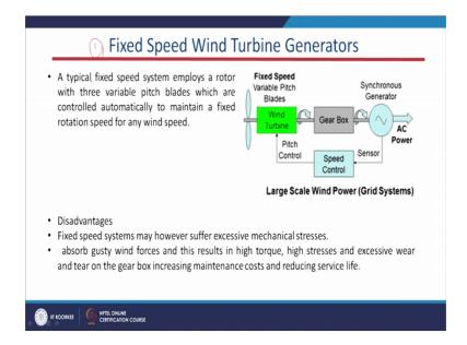
The first one is fixed speed wind turbine generators and, in this case if we will see this one it is a large scaled wind power and it is a grid system here, it is the wind turbine.
