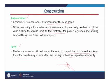
Now, this anemometer is also there it is a basically sensor, which measures the wind speed here, it is it measures the wind speed and it is further it is used for our controlling purpose only, it is a feedback it will be a feedback to the controller. And for rain resource assessment it is normally fixed on the top of the wind turbine.
