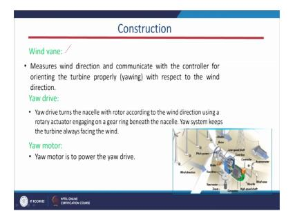
And this is our wind vane basically the it is an equipment, which is present inside the wind system, here it is if you will see this figure this is our wind vane. And this wind vane measures the wind direction it a does not measure the wind speed the wind speed is measured by this anemometer.
