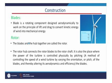
Coming to the blades of the wind fan so, this structure a this is a this is our blade of the wind energy system. What is the function of this blade? This blade is a rotating component which is designed arrow dynamically to walk on the principle of lift and drag, this is important, drag to convert the kinetic energy into the mechanical energy.
