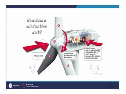
Then come to the principle of operation of the wind system, that is a very simple picture I have kept, this A and B together called as the rotor of the wind system. And this is the flow of the wind, the first stage is the flow of the wind and second this second stage, in flow of wind activates the rotor and blades. This A stands for the rotor and this B is the blade.
