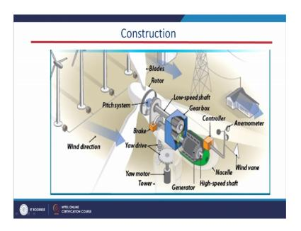
The first one I will just talk about the rotor and the blades. And second system is the pitch, third one we have the low speed shaft then we have gear box, then we have high speed shaft and, then we have generator, then we have controller and of course, we have this breaking system and yaw drive and yaw motors and then the tower.
