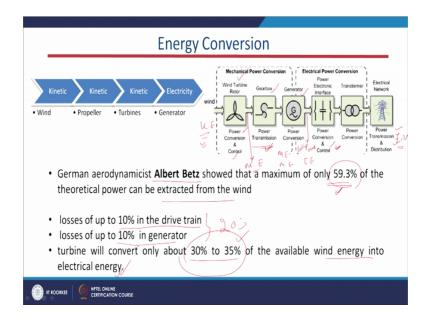
And these are some of the stages these are the block diagrams, the first stage the power energy conversion part is there, as well as the wind turbine rotor is concerned, at the wind turbine rotor section will have the power energy conversion. What is that type of power energy conversion? The input will be the kinetic energy, the output will be mechanical energy.
