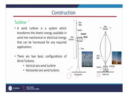
It will come to this figure this is our horizontal blade, or horizontal tower of the wind system, and this is our vertical wind system. What is the difference between these two? The first difference is that in case of horizontal based type of wind system, here the generator and the gear box are mounted on the top of the tower, or top of your this system this is our tower. But in this case the generator gear box are mounted on the bottom.
