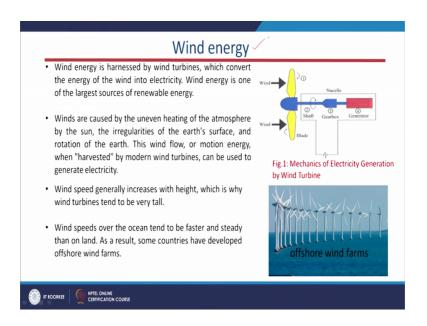
Now, I will just discuss here what is this wind energy; if you could see here this figure so, it is schematic figure of this wind energy system, where I have shown this two arrows basically the wind flow, flow of the wind system wind and this is our blades these are the blades and, we have shaft and gear box and the generator.
