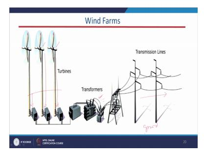
Now, this is a very typical wind farms picture here, our wind turbines and we have the generator basically the here, it is the this is a nacelle section, where the generator is present and from there we will take out the electrical power.
