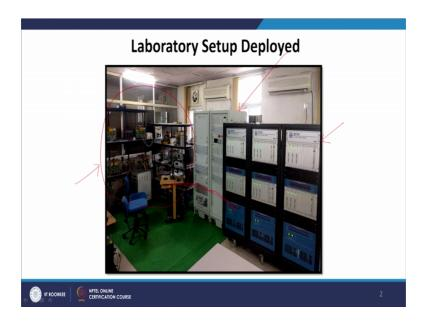
Now, this is how actually the lab look like so, I mean you can just see that is. So, this is mainly the RTDS of 6 rack and we can say this is the power amplifier, and then we have the smart grid hardware test bench. Now, all the 3 that is RTDS power amplifier and the test bed on smart grid being connected and simulated simultaneously. Now, let us understand what are the devices currently available in the laboratory smart grid laboratory?
