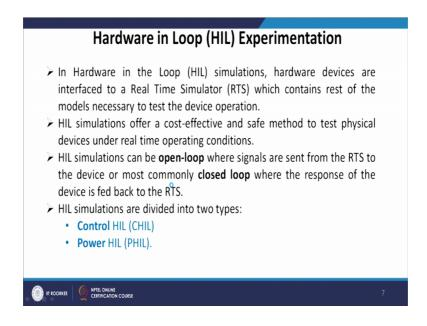
And, in hardware in loop HIL simulation hardware devices are interfaced in a real time simulator that is RTS, which contain rest of the model necessary to test the device operation. So, through HIL we basically connect the hardware devices to your simulator and most of the components are available within the simulator and few hardware devices that can be interfaced with your simulator.
