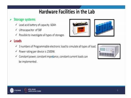
Now, we also do have storage sources and lead acid battery of capacity, 60 ampere hour and then we have ultracapacitor of 58 farad and we can possibly investigate all type of storages. And, we do connect approximately the given time maybe if, 6 to 8 kilowatt of or the KVA of storage that can be connected to my test bed at any given time through battery.
