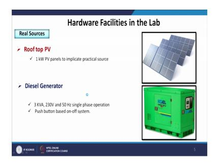
So, if you see the sources is as high as actually 4 kilowatt of PV and 2.2 for wind. And, 1 4 rooftop and 3 4 diesel so, close to 10 kilowatt source has been connected to the test bed. So, I can say it is a interesting setup which is very nicely handle 10 kilowatt capacity.
