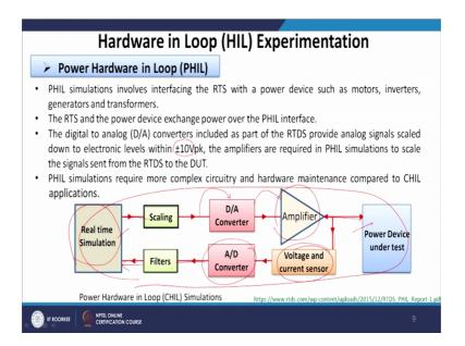
In case of Power Hardware In Loop simulation PHIL simulation involves interfacing the simulator that is RTDS with a power device such as a motor, inverter, generator, and transformer. And, the real time simulator and the power disk device exchange power over the PHIL interface.
