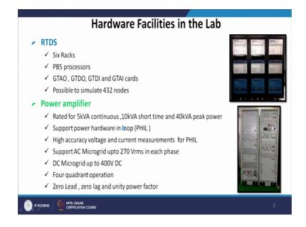
So, the hardware facilities available in our smart grid lab we do have a RTDS, which is of 6 racks, PB 5 processor, GTAO based, GTDO based, GTDI and GTAI card based RTDS. And, the very important part the RTDS can simulate a system which is a maximum of 400 and 32 nodes.
