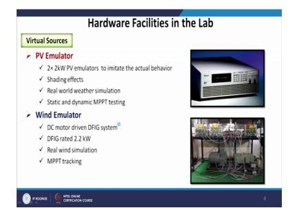
Which, will mimic your solar PV and we have connected 2 2 kilowatt PV emulator to imitate the actual behavior of APB solar, it has the capacity to accommodate the shedding effect, real world whether simulation is possible, static and dynamic MPPT testing also can be performed with the simulator.
