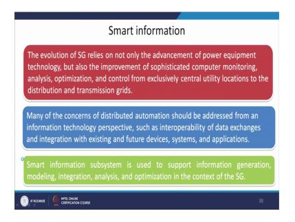
Now, many of the concerns of the distributed automation should be addressed from an information technology perspective, such as interoperability of data exchanges and integration with existing and future devices, systems, and their applications. Smart information subsystem is used to support information generation, modeling, integration, analysis, and optimization in the contest of the smart grid.
