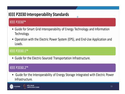
I triple E P 2030 Interoperability Standards I triple E P 2030 guide for smart grid interoperability of energy technology and information technology, operation with electric power system and end use applications and loads.
