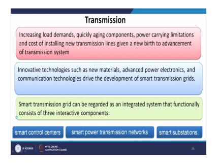
Now, the transmission defines as based on the increasing loads demands, quickly aging components, power carrying limitations and cost of installing new transmission lines given a new birth to advancement of transmission system.
