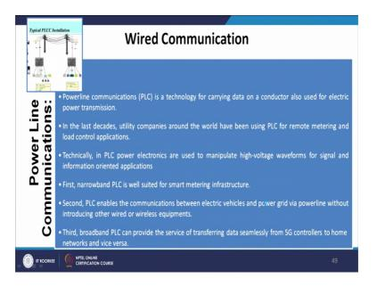
Power line communication that is PLC is a technology for carrying data on a conductor also used for electric power transmission. In the last decade utility companies around the world have been using PLC for remote metering and load control applications.
