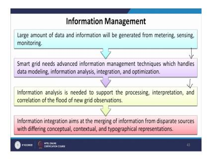
Now, and hence we have to manage the information, the information management is being carried out through, different steps large amount of data and information will be generated from metering, sensing, and monitoring, through different equipment and devices and those will be passed through smart grid, that needs advanced information management technique, which handles data modeling, information analysis, and integration, and optimization.
