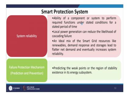
Smart protection system achieves system reliability that is ability of a component or system to perform required functions under stated conditions for a stated period of time. Local power generation can reduce the likelihood of cascading failure an ideal mix of the smart grid resources like renewable demand response and storage lead to flatter net demand and eventually increase system reliability.
