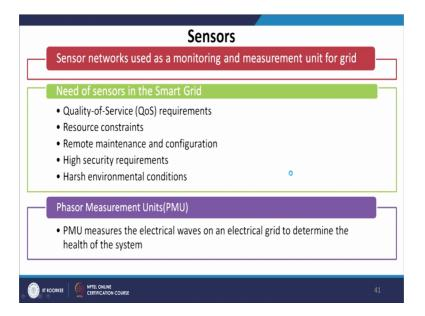
Censor networks used as a monitoring and measuring a unit for grid need of sensor in the smart grid is mainly; because of it is quality of service, resource constraints, remote maintenance and configurations, high security requirements, harsh environmental conditions. Now, one more important point here I like to emphasize that we need to have phasor measurement units that is PMUs PMU mainly measures the electrical waves of an electrical grid to determine the health of the system.
