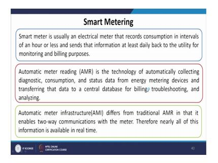
Automatic meter reading very commonly known as AMR system is the technology of automatically collecting diagnostics, consumptions, and status data from energy meters and transferring that data to a central database for billing, troubleshooting, and analyzing.
