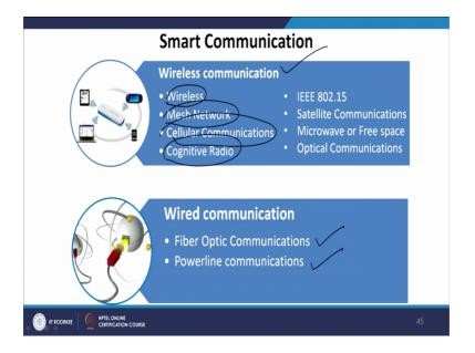
Smart communication we can see one of the major smart communication is wireless communication, it has wireless mesh network, cellular communications, cognitive radio, and these wireless communication is quite important for successful operation of a smart grid. Now, when we talk about wired communication they could be either fiber optic communications or it could be power line communications.
