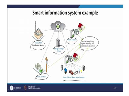
Now, if you look at smart information system example. Now, first of all this is the utility and we do have energy storage devices in place, and then we have the smart meters and then the smart routers are placed and the smart meter home area network is through low cost Zigbee metering communication devices are placed for the exchange of information within smart grid.
