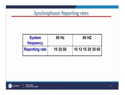
And this is the synchrophasor reporting rate this is for 50 hertz, 10 samples per cycle; 25 here, 50 here and for 60 hertz these are the figures this is IEEE standard basically. And this is the basically the file structure of synchrophasor standard.
