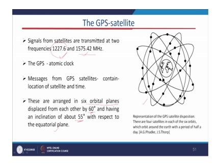
And this GPS already we have discussed that GPS transmits basically two frequencies; the first one is 1227.6 and second one is 1575.42 mega hertz. So, this two frequencies are the transmitted frequency by the GPS technology and if you will see that there are these are arranged in 6 orbital planes and displaced from each other by 60 degree and having a inclination of 55 degree with respect to the equatorial plane.
