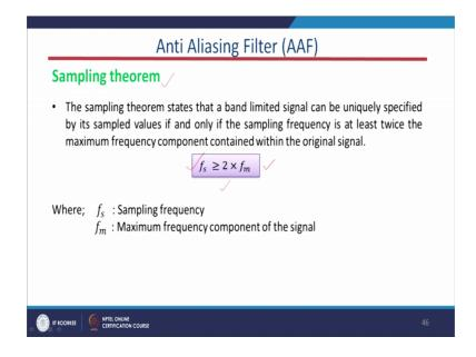
This anti aliasing filter; first we maintain one theorem that is sampling theorem and Shannon's theorem; what we have to do? We have to maintain the sampling frequency in such a manner that it should be greater than twice of the higher frequency component of the signal. Let us say we have certain high frequency component which is present in a particular signal. So, our sampling frequency should be two times of that particular signal it should be greater than that or equal to that.
