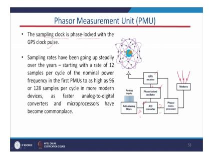
Now this if you see this PMU gets this clocks all this sampling clock is phase lock with the GPS clock pulse; this is very important. This phase locked oscillator and the GPS clock together they are locked, then only this ADC will start converting; I mean sampling this analogue signal to digital domain. It will just start sampling this analogue signal to digital domain.
