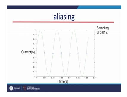
This aliasing effect means if a fundamental basically we have let us say 50 hertz signal, but during the power system operation; we have like higher fundamental higher frequency components like other harmonic frequency components, second harmonic, third harmonic, fourth or 5th harmonic components are present; so those are higher frequency components.
