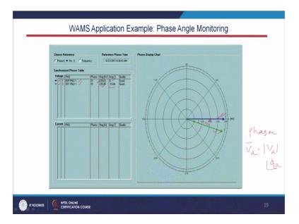
This is one snap shot that WAMS application for phase angle monitoring that you could see here that there are two buses two buses. So, we have placed PMU 1 and this 2; so, for that particular one PMU; the voltages and magnitude is 239.63 and angle is 0 degree and this is the phasor position. If you could see in this will this circle and here the second part the voltage let us the magnitude is 235.84 and the angle is minus 15.0 degree and here is the phasor positions.
