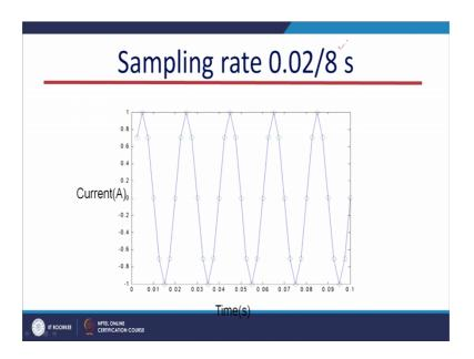
That is 0.02 by 8 means 8 samples per cycle and in that case; you can see here the signal is not approximated at to actually to our actual signal, the approximation is less here. You can see here it is better because we are just taking more number of samples within 1 cycle, but here the number of samples decreased that is why the approximation of the exact signal is not possible. Now if we will increase the number of samples per cycle more like here we have taken 64.
