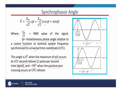
So, these are the concepts of Synchrophasor angle measurement; so this 1 pulse per second, 1 PPS corresponds to this t equal to 0, when this cosine function is having the peak value. This is what the definition by the IEEE standard that how to standardize this synchronized angle; universally this angle should be synchronized.
