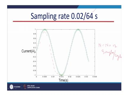
N we denote capital N; N basically stands for number of number of samples, samples per cycle. So, if we have increased here the number of samples per cycle to 64. So, in that case we have better resolution better approximation to our original signal. That means to have a better approximation or exact if you want to extract or we want to convert the exact analogue signal to digital. That means, we have to increase the sampling frequency.
