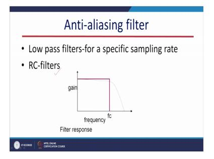
Now, also we maintain low frequency like low pass filters where will just remove the higher frequencies and will just passed the low frequencies and also our fundamental frequency for our application purpose. Basically in this case we use the RC filters and sometimes we you can see that some other low pass filters are also used.
