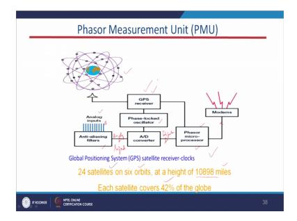
This is basically the basic block diagram of the PMU; we have first the analogue inputs the analogue inputs means the voltage current signals. And these voltage current signals will pass to the anti aliasing filters. We will discuss about this; what is the function of this anti aliasing filter. Then it will go to the ADC converter the data and here still this is analogue this signal is analogue here.
