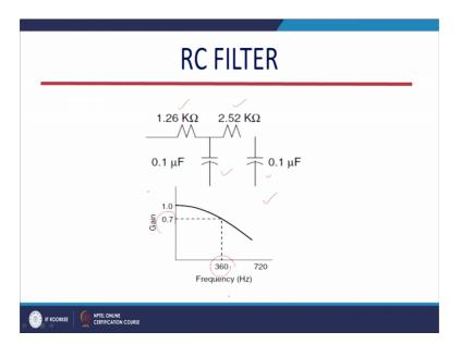
Now, this is one specific example where the RC filter is shown that these are the resistances values and these are the capacitance values and this is how this gain here present and this is how 360 is the cutoff frequency. So, there are lot of resource is also
