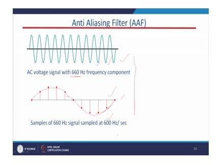
That this particular waveform is having 660 hertz frequency component and if you are just sampling this particular waveform at a rate of 6000 hertz per second. So, we will get the signal like this here.
