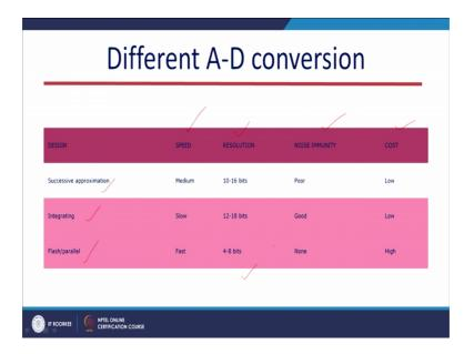
And we have different type of ADCs like successive approximation integrating flash or parallel. So depending on their resolution, speed and also noise immunity and cost; so this is a table how this particular all different types of AD: ADC vary in their operation.
