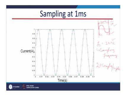
If we have voltage waveform then for riling purpose for protection purpose, the sampling rate is basically safe side we took basically 1 kilo hertz; 1 kilo hertz, that sampling frequency we denote by f s; this f s is known as sampling frequency. Now if this sampling frequency is 1 kilo hertz and we have a 50 hertz signal let us say voltage signal.
