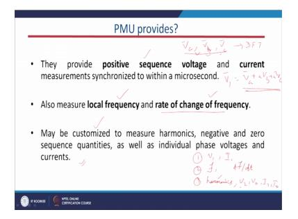
Basically among question comes here that what are the data or voltage information which are provided by this PMU? This PMU provides positive sequence voltage and current also now; if we have inside the PMU we have discussed that we measure or we estimate this voltage like V a maybe V c phasors using the DFT; the Discrete Fourier Transform technique. By using this phases; so we can always calculate the positive sequence component of the voltage that is V a plus a V b plus a square V c.
