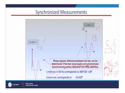
Now, I will just come quickly the again to this PMU part how it measures the synchronized data; synchronize the synchronized phasor, voltages and currents. Now this is one location in the network, this is location 2 that these two locations are apart from
