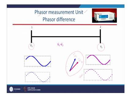
And. In fact, this PMU is the heart of our wide area monitoring system. So, without this PMU the wider area monitoring system has no meaning. So, this PMU stands for Phasor Measurement Unit and basically as the name suggest that phasor; it measures the phasor of the voltage and current. If let us say these are two busses where we have this V 1 is the voltage magnitude or phasor of bus 1 and this V 2 is the voltage phasor for bus 2.
