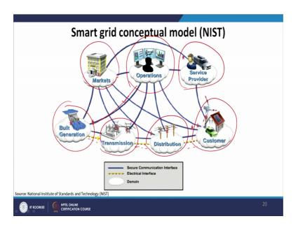
Now, the NIST National Institute of Standards and Technology provides you the pictorial view of how the smart grid conceptually works? Now, we can see there is bulk generation and we have transmission, then distribution, and customers.
