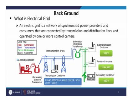
The moment we talk about electrical grid, it means electric grid is a network of synchronized power providers and consumers that are connected by transmission and distribution lines and operated by one or more control centers.
