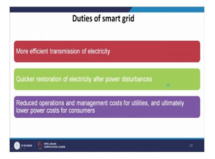
Now, the major duties of smart grid is more efficient transmission of electricity quicker restoration of electricity of after the power disturbances, reduced operation and management cost for utilities and ultimately lower power cost for consumers.
