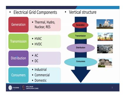
Now, the different components of electrical grid to me is generation first, which is either of thermal type, hydro type, nuclear type, and very recently renewal energy sources. Now, the transmission has being told a recently it is either of high voltage AC or high voltage DC, the distribution system mostly it is AC type, but in the recent time people start to talking about DC type too.
