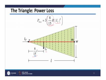
And from this expression, you can easily find out location of your lump load. So, from this we can see that at 8 by 15th distance, or resistance value of 8 by 15th, I can lump total current. So, total current will be lumped at 8 by 15th distance.
