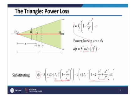
Now, let us see the power lose equation so, current equation, which we have derived which is entering into the strip, which is given by these equation we already seen it. Then power loss which is happening in this small strip will be nothing but 3 into resistance of the strip which is r dx and current in thing into the strip which is i square.
