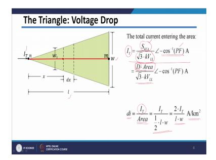
So, let see the voltage drop first. So, if you know the total kVA, we can easily get the current which is entering to this particular feeder, which is given by these equation here, which is just your kVA divided by root 3 times your line to line voltage. And then there is cos inverse of power factor where this power factor is average value of power factor over your distribution area.
