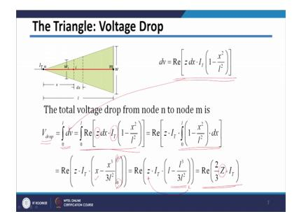
So, to get total voltage drop across the feeder or till the end of the feeder, we need to integrate this dv from 0 to 1. So, total voltage drop across the feeder will be integration of this dv from 0 to 1, equation of dv we obtained it here I can put into this expression I will get this equation here, and in this case also your z and I T they are constant, I can take it out remaining term they will be get they will be getting integrated.
