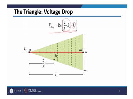
So, from this equation we can easily find out, the lump load model of triangular configuration. So, this is your voltage drop equation and, I can see that this 2 by 3 into Z total Z multiplied by your, I T.
