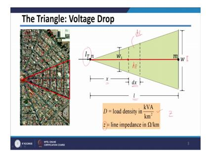
In this case consider this a triangle area here, we can assume that substation is somewhere here, and then there are actually primary feeder which is going in this area. And then there will be laterals which are connected to the primary feeder and, this laterals are supplying power to the various consumers, which are inside this particular area.
