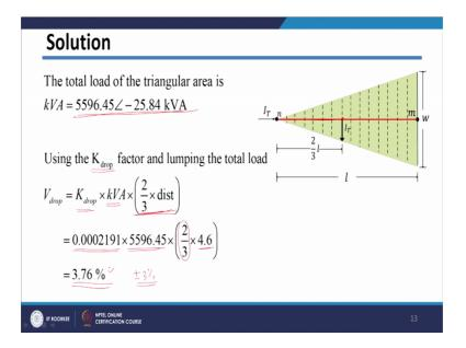
Let say let see how we can find out this location here. So, total load of triangular area which we have calculated on the last slide is given here. Now, using K drop factor we can calculate actual drop without capacitor. So, actual drop so, K drop factor we know that kVA percentage drop per kVA per kilometer. So, if you can multiply this K drop factor by kVA and kilometer, we can get voltage drop
