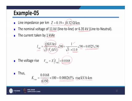
Let us say impedance of your line is Z is equal to 0.19 plus j 0.32 ohms per kilometer. Nominal voltage of your feeder is 11 kV therefore, phase to neutral voltage or line to neutral voltage will be 6.35 kV. And in this case we want to calculate current taken for 1 kVAr load because we want to calculate K rise factor which is basically percent voltage drop per kVAr per kilometer. So, to get current per kVAr we need to calculate current for
