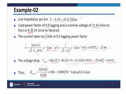
Let us see for a simple feeder, how can we calculate this K drop factors. Let us say you are having impedance of the feeder which is given here, Z is equal to 0.19 plus j 0.32 ohms per kilometer which is impedance per kilometer. Let us say power factor of the load is 0.9, nominal voltage of the feeder is 11 kVA line to line, in that case your line to neutral voltage will be 6.35 kV then current taken by 1 kVA at 0.9 lagging power factor.
