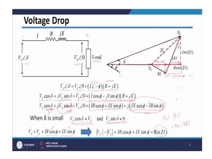
Let us see this figure what I have done it here you have this feeder component from say point 1 to point 2, which is having resistance of R and reactance of jX. And then there is load which is having say lagging power factor voltage at load end is actually V L angle 0 and voltage at sending end say V S angle delta
