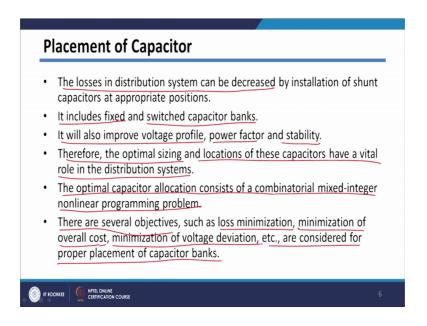
Next thing we have seen that placement of capacitors is also planning problem, because we are considering the placing the capacitors in the distribution system. So, first we need to calculate, how many capacitance we know need, what are the location, where the suite where the capacitors can be placed. So, this new location should be optimal.
