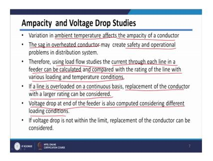
Then third is ampacity and voltage drop studies. Ampacity is nothing but current carrying capacity of your conductor. However, these current carrying capacity depends on ambient temperature. So, whenever temperature increases, your resistance of the conductor changes, or increases, and because of that resistance your ampacity decreases.
