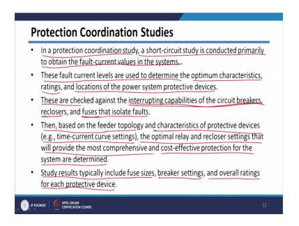
And then, we have seen the short-circuit analysis also. Let us see, what are the applications of the short-circuit analysis. So, main application of short-circuit analysis is protection, coordination, studies. So, in a protection coordination study, or short-circuit study is conducted primarily to obtain low fault-current in the system. So, we have seen various methods based on which we can calculate fault currents in the distribution system.
