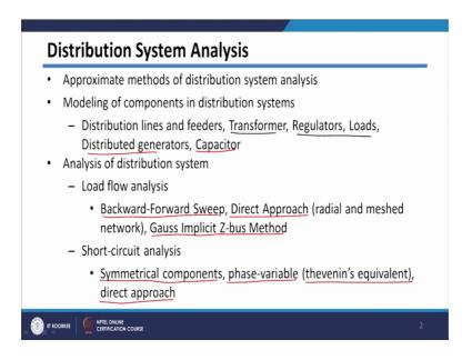
So, basically we have seen various methods of distribution analysis starting with approximate methods. So, in approximate methods, we are actually approximated your distribution system. And using the simplified models of distribution system, we try to calculate voltage drops, and power loss in the distribution system.
