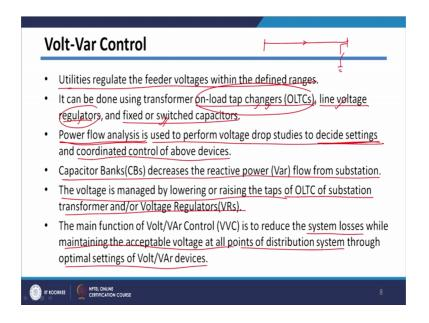
Another important operational issue is volt-var control. So, we know that utilities regulate the feeder voltages within the limits. So, we have we have seen that standard specifies at various countries, standard specifies these limits of voltages. So, voltages of the distribution system should be vary within that limit. There therefore, I have written utility regulate the feeder voltages within the defined ranges.
