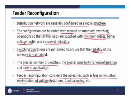
Next problem is actually distribution reconfiguration, or it is also called as feeder reconfiguration. We know that these distribution networks are generally radial in nature. And if you can provide switches at various lines in the distribution system, and if there
