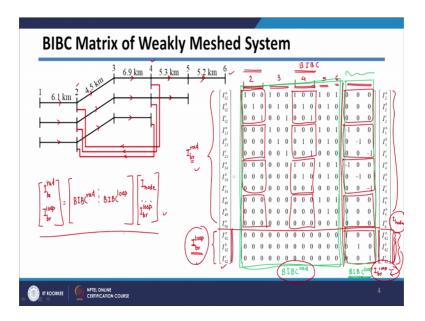
Now, in case of weakly meshed system, let us consider this system here. So, here I am considering one there is one line, which is meshed one. So, here the black one is radial system. However, there is one line, which is meshed, which is carrying current into this direction. So, here in this case currents are actually I am considering line currents, which are in this direction; And through this meshed branch, the currents in this direction.
