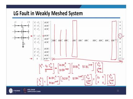
So, by replacing these entries, so we have basically replace this entry here. And these two entries, which are non-zero, other entries are 0 here. So, in this case to get the fault current value, what we can do, we can just consider this expression here, or only this row.
