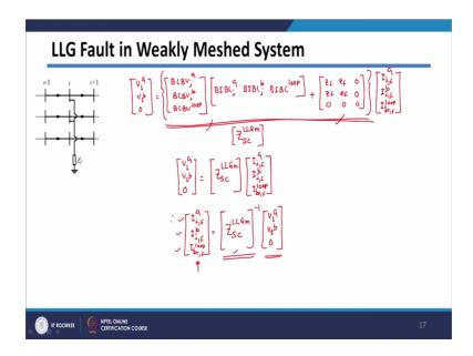
So, in this case, I can just write it like this. So, it will be V 1 a V 1 b 0 will be equal to BCBV corresponding to a, BCBV corresponding to b, BCBV corresponding to loop forming branches, which will get multiply with BIBC corresponding to a phase, BIBC corresponding to b phase. And BIBC corresponding to loop forming branches plus Z f Z f 0 Z f Z f 0 0 0 0, and the term which is taken out common is fault current in a phase, fault current in b phase, and fault current in loop forming branches.
