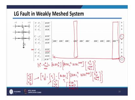
So, in generalize sense, I can easily write. So, in generalize sense, I just erase this here. So, I can write V j will be equal to V 1 minus BCBV of j multiplied by this term will remain common same, BIBC of a phase, BIBC corresponding to loop forming branches, and this will get multiply with fault current in a phase, fault current in loop forming branches.
