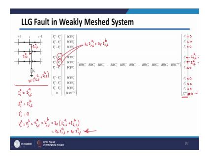
Now, let us see how we can consider LLG fault in weakly meshed system. So, in case of LLG fault, there are two buses, which will be faulted with ground. So, here I am considering phase a, and phase b, which is faulted with respect to ground. So, let us say current in a phase is post fault current in a phase, and current in b phase is post fault current in b phase.
