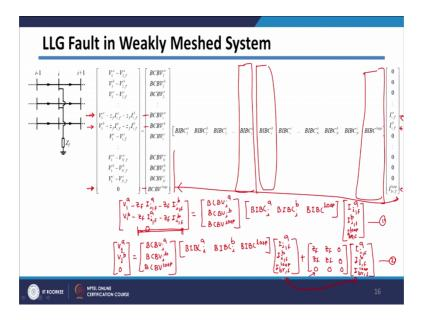
So, these corresponding entries I have just replaced in this row, and corresponding currents I replaced in this column here. So, except these two currents, i and b, and branch currents in loop forming branches, all other currents are 0. So, from this to write your fault current equations for LLG fault in weakly meshed system, we need to consider these three types of rows; So, these two rows, and rows corresponding to your loop for being branches.
