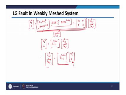
So, I can rewrite this equation like this. So, on this side it is V 1 a 0, which is equal to BCBV corresponding to loop forming branches, which is getting multiply with BIBC corresponding to a phase, and BIBC corresponding to loop forming branches plus Z f 0 0 0. And since we are taking common out from both the terms; so, it will be I fault current in a phase, and loop forming branches.
