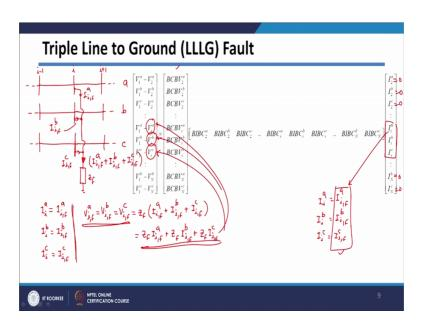
Now, let us see a triple line to ground fault. And in case of tipple line to ground fault, the ground fault occurring three phase to line three phase to ground. So, let us say, in this case also let us considered any ith bus, so this is will i plus 1th bus, this is say i minus 1 bus. So, this is say corresponding to a phase, then corresponding to your b phase, and this is corresponding to c phase.
