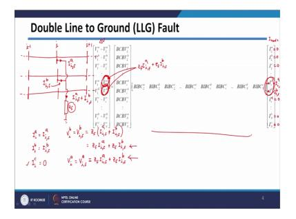
And we are going to use them for short-circuit analysis. And as I told you in last class, we have studied single line to ground. Let us start with now double line to ground fault here. So, in this case, again consider any general bus, say this is ith, bus this is i plus 1, and say i minus 1 bus. And since it is part of large system, I can just show it is other
