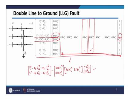
These two currents, and modifying these two entries to post fault voltages, we will basically get this matrix. So, as explained in earlier slide, I just modified these two entries here, and these two entries here, and these entries I just post fault voltages I have
