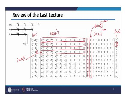
So, in particular in the last class, we have seen that using your direct approach based method. We can write this equation, which is basically delta V, which is equal to your BCBV matrix, which is having structure like this contains impedances. And then this is
