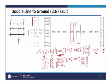
Similar way, generalize way if you want write the voltage equation using whatever we have done in case of LG fault, I will just write them here. So, it will be V j post fault will be equal to V 1 minus BCBV corresponding to any jth bus, where we want to calculate post fault voltages, and this will get multiplied with respect to BIBC. Either shown you only these two columns are getting multiplied with respect to fault currents, and multiplied by your fault currents sorry this is fault current.
