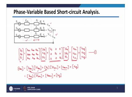
So, let us write the equation for this. So, if you write the kvl equations for this particular figure here. So, I can easily write on the right hand side, there will be sources. This is E a, E b, and E c, the voltage will be equal to the impedance drop across this impedance say that is Z abc Z abc.
