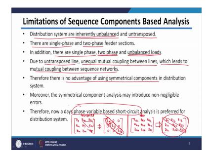
So, we have seen that we distribution system is inherently unbalanced and untransposed. And as we have seen that in case of sequence component theory one basic assumption is that system is balanced before fault and only positive sequence quantities exist in the network before the fault. So, that condition will not be get will not get satisfied in case of distribution system because distribution systems are very much unbalanced before fault also.
