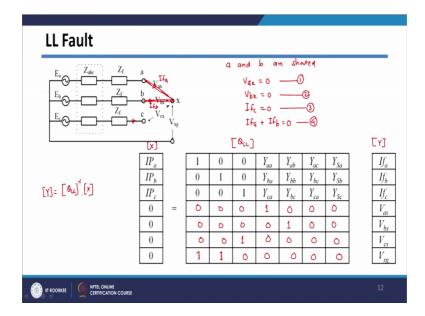
Let us consider one more fault LL fault. So, in this case say line a and b are shorted. So, in this case say a and b are shorted means this will be shorted with respect to this line. So, I can say V ax will be equal to 0; V bx will be equal to 0; I f c will be equal to 0, because there is not be current it is not faulted. And one more equation which we need that I can get whatever this current I a will be opposite of I b.
