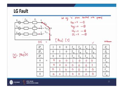
So, we have got this circuit matrix here. And if you are considering LG fault, so in case of LG fault let us say you are a four a phase is faulted; so in this case since with ground. So, in that case, your a phase and this will be grounded ok. So I, in that case I can say V ax will be equal to 0; there will be as well as V xg will be equal to 0.
