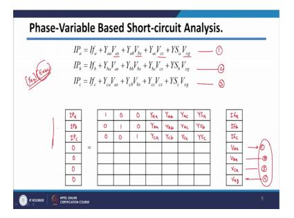
Now, if you write these equations, so we have got this relation here which is basically IP a IP b plus IP c is equal to I f a I f b and I f c plus your y metrics that is Y aa Y ab Y ac Y ba Y bb Y bc Y ca Y cb Y cc multiplied by your voltages V ax V bx and V cx plus as we have seen that this part we have converted into V Sa into YSa into V xg Y Sb into V xg Y ac into Vxg. So, it will be Y sa into V xg Y s b into V xg and Y sc into V xg.
